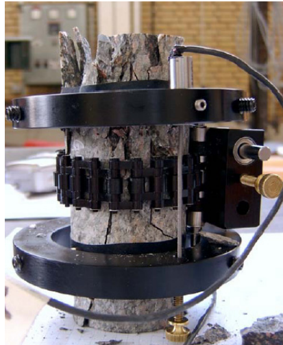
Figure 53. A rock specimen on completion of the complete stress-strain curve testing in uniaxial compression. Åspö diorite rock core sample; SP Laboratory, Borås, Sweden (Hudson 2005).
