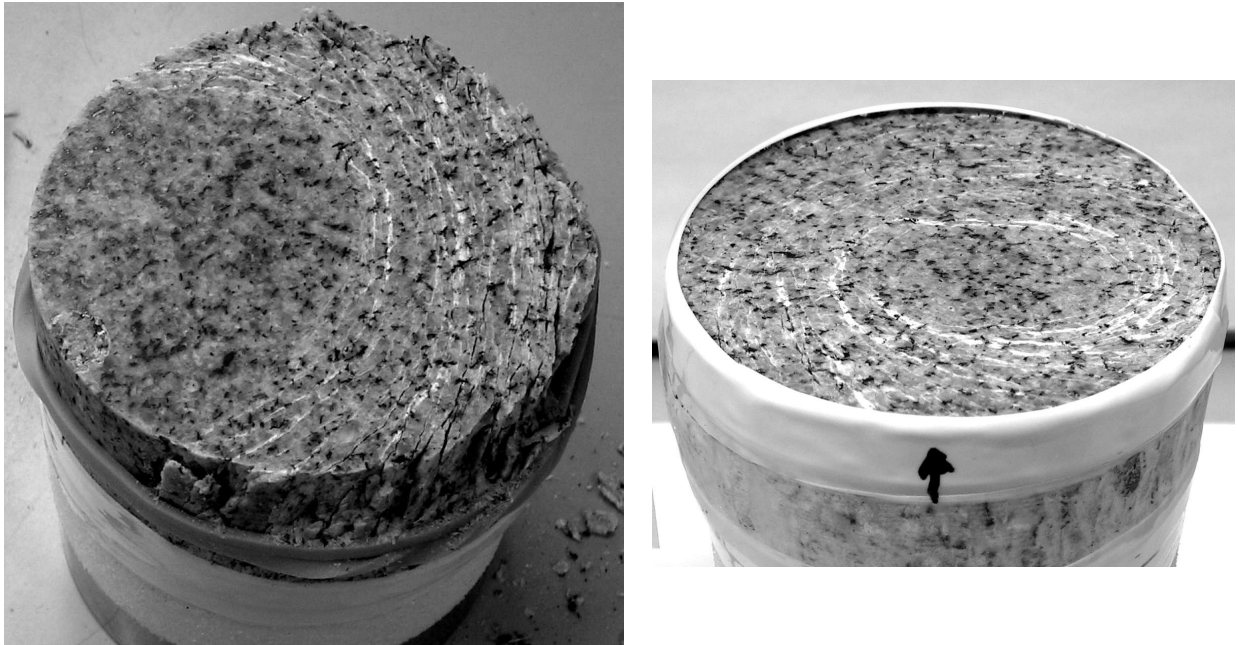
Figure 44. Gradual failure of specimens 5A (left) and 9B (right).
