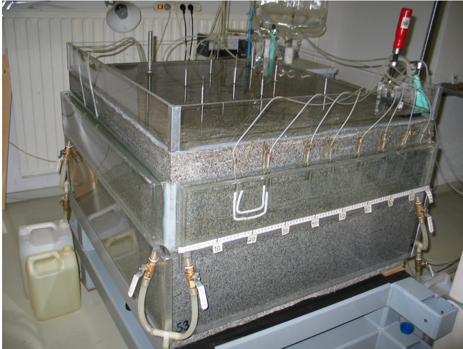
Figure 91. The experiments were carried out in the horizontal natural fracture located in the upper part of the rock block. Water pools installed on the vertical faces of the rock block are used to apply appropriate boundary conditions to the outer boundary of the fracture.
