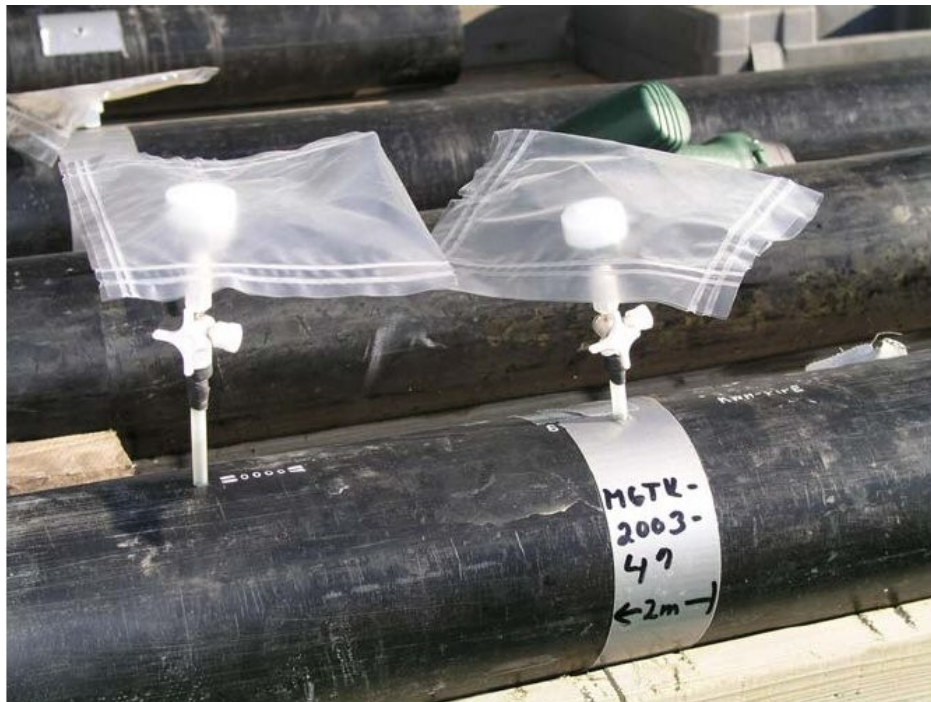
Figure 80. Additional gas samples taken from a sediment core (Photo Jyrki Hämmäläinen).
