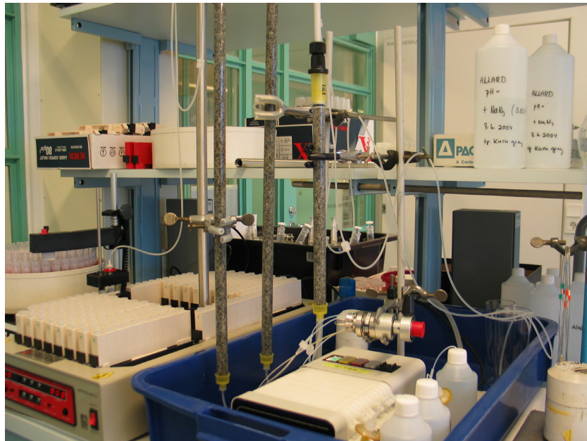
Figure 89. Experimental design used in rock-core column experiments. Cores drilled to the fracture of the Kuru Grey granite are placed inside a tube to form 74.5-cm-, 68.5-cm-, and 28-cm-long columns. Core diameter is 14 mm and flow channel is in the 0.5 mm gap between the core and the tube.
