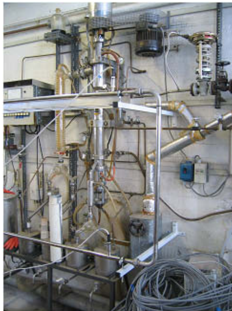
Figure 5.33. Flow elbows and pressure sensors Pt107 and Pt108.
