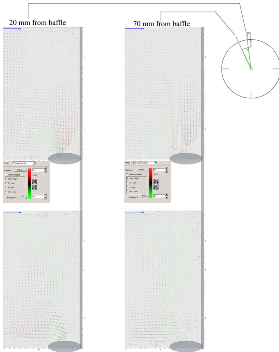
Figure 2.15. PIV measurements of water in crystallizer. Mixing velocity of propellers was 385 rpm. Color of the vectors describes the third dimension in right handed coordinates.
