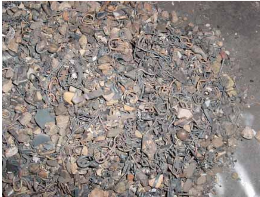
Figure 6. Coarse fraction of the bottom ash at set point CFB 05/05B.
