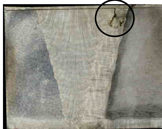
Figure 96. Examples of defects manufactured by techniques “A” and “B” after destructive examination (Eriksen et al. 2004).
