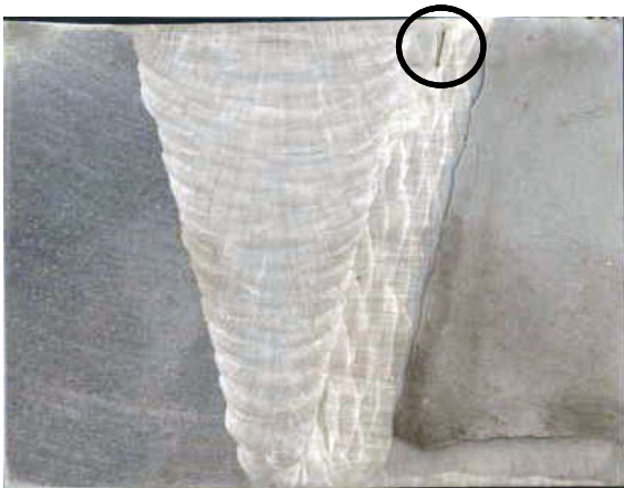
Figure 96. Examples of defects manufactured by techniques “A” and “B” after destructive examination (Eriksen et al. 2004).
