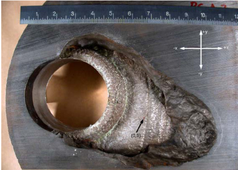
Figure 76. Picture of the corroded Reactor Vessel Head at Davis Besse (NRC Operational Experience).
