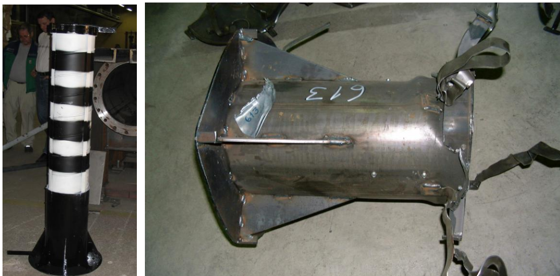
Figure 100. Spiral-weld steel pipe missile before (on the left) and after (on the right) the test.
