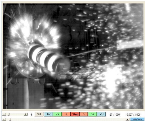
Figure 98. Still figures of steel pipe missile during an impact.
