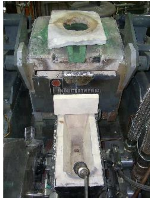
Figure 112. Top view of the induction furnace and vessel with melt flow path opening for melt.
