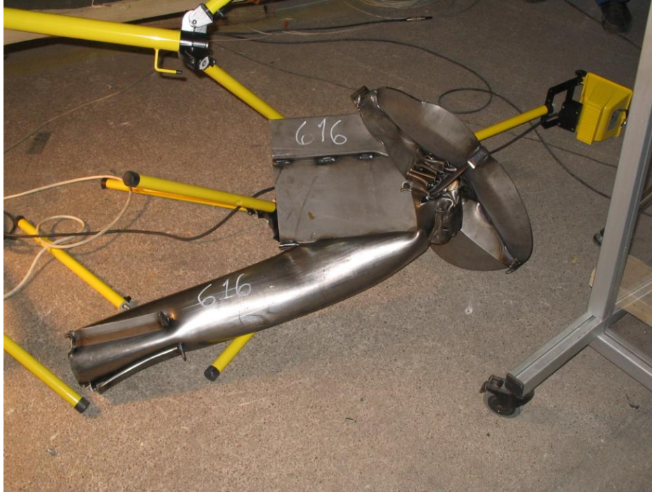
Figure 96. Steel piston after impact with the speed of 143 m/s.
