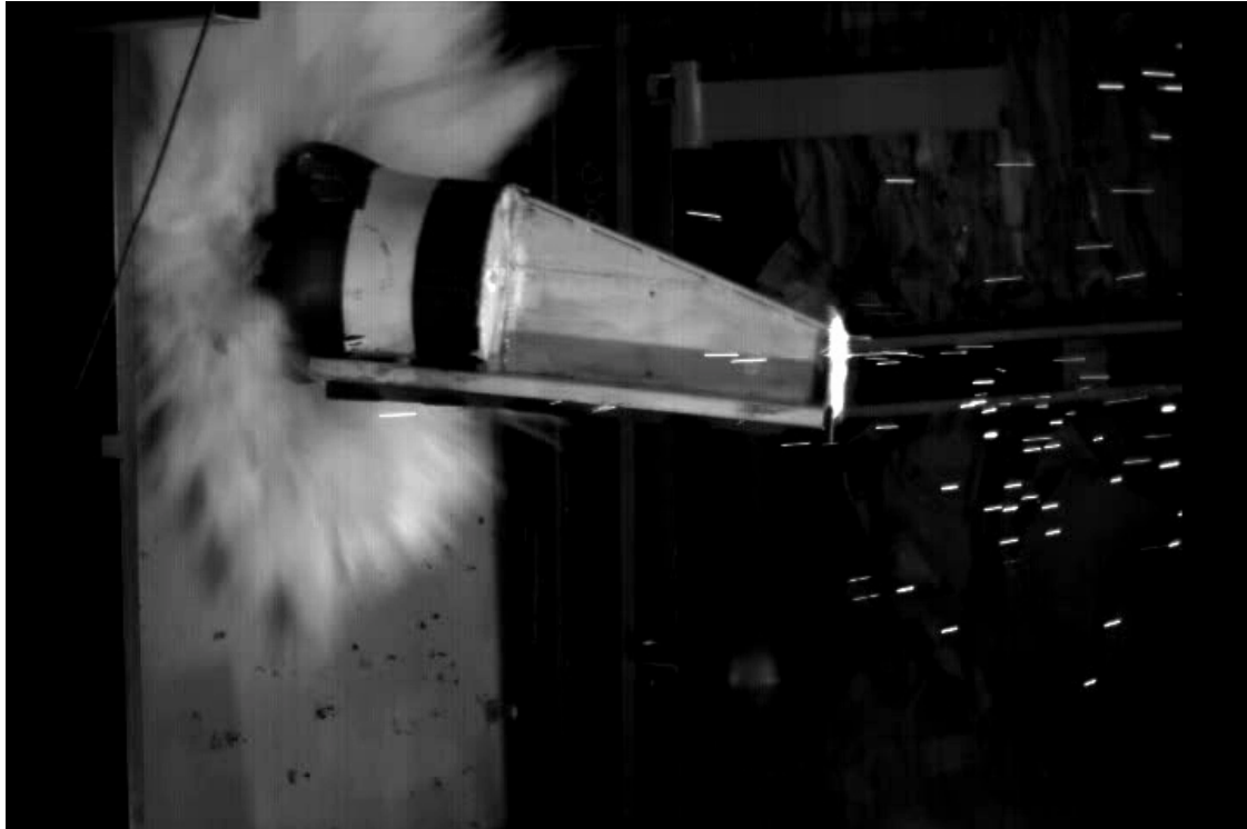
Figure 104. A still figure of impacting steel pipe missile filled by water.
