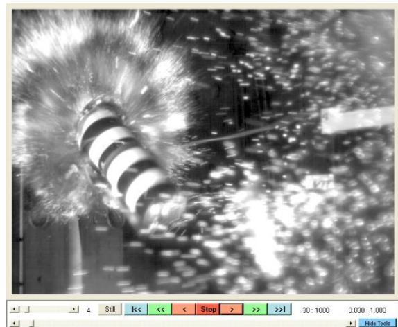
Figure 98. Still figures of steel pipe missile during an impact.
