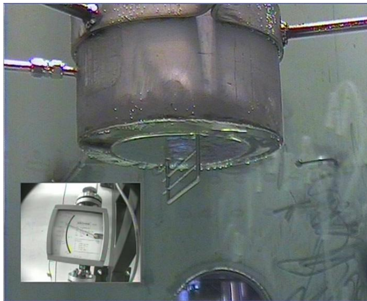
Figure 93. Stable steam-water interface at blowdown pipe exit in POOLEX test for NURESIM.
