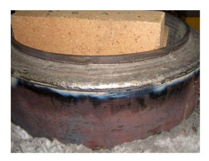
Figure 2.201. Pressure vessel steel pipe after first buttering layer.
