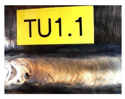
Figure 2.50. Root side surface of the test piece in mock-up 1 with hot cracks after Varestraint test. Augmented strain was 4%.
