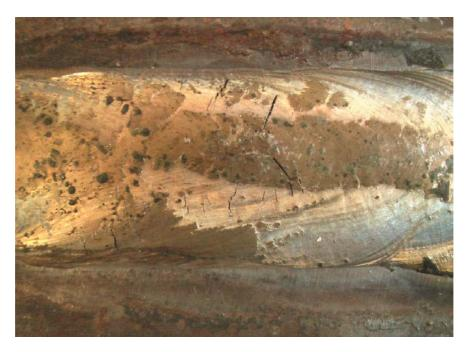
Figure 2.29. Surface of the test piece with hot cracks after Varestraint test. Augmented strain was 3%.
