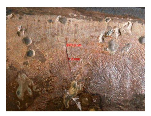
Figure 2.37. Measured crack lengths with magnification of 25x. Augmented strain was 1%.
