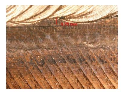
Figure 2.47. Measured crack length in TV test piece with magnification of 25x and augmented strain of 2%.
