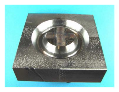
Figure 2.188. The ring segment test specimen after tack welding and machining of circumferential groove.
