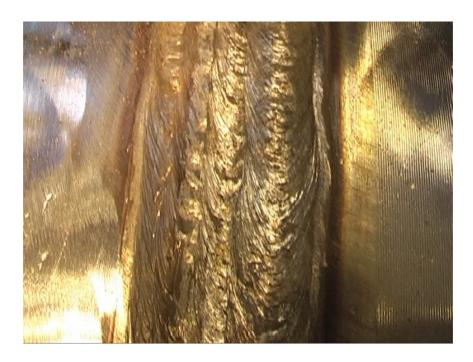
Figure 2.212. Surface of the Neste Oil dissimilar metal weld mock-up after welding.
