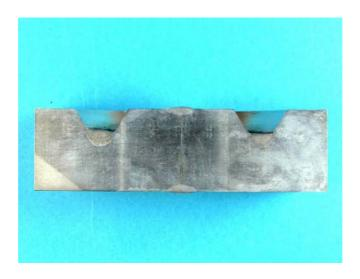
Figure 2.194. Cross-section of the Inconel 182 test specimen.
