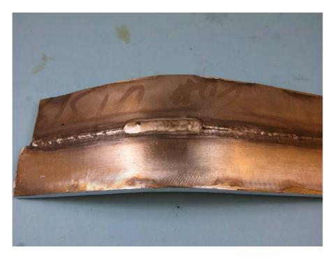
Figure 2.40. Test piece TV after Varestraint test. Augmented strain was 4%.
