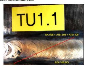
Figure 2.154. Cutting line of cross-section of mock-up 1 sample for microstructural examinations after Varestraint test.
