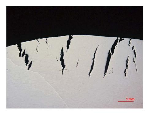
Figure 2.104. Cross-section of Neste Oil weld cracks after Varestraint test.
