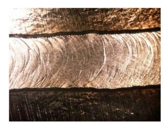
Figure 2.76. Test specimen of Inconel 82 weld after testing with 4% augmented strain.
