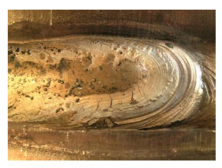
Figure 2.33. Surface of the test piece with hot cracks after Varestraint test. Augmented strain was 2%.
