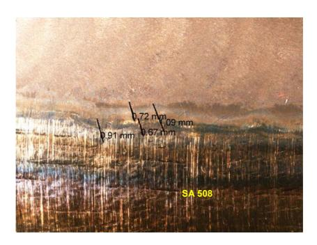
Figure 2.68. Measured crack lengths in mock-up 3 with magnification of 25x and augmented strain of 3%.
