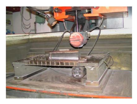
Figure 2.5. Wire Electro Discharge Machining (WEDM).
