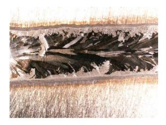
Figure 2.81. Test specimen of Inconel 52 weld after testing with 4% augmented strain.
