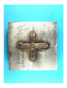
Figure 2.187. Ring segment test specimen after tack welding.
