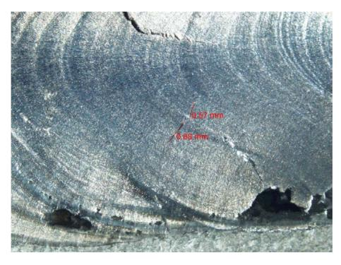
Figure 2.43. Measured crack lengths in TV test piece with magnification of 25x. Augmented strain was 4%.
