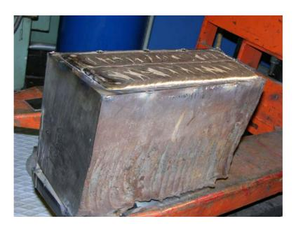
Figure 2.10. First layer of cladding on pressure vessel steel SA 508 Grade 2.
