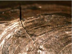
Figure 2.195. Crack 1 in Inconel 182 weld. Figure 2.196. Crack 2 in Inconel 182 weld.
