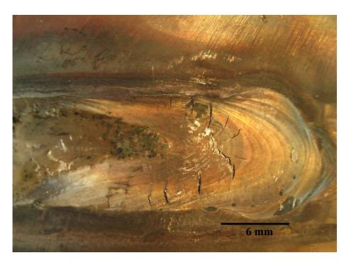
Figure 2.23. Surface of the test piece with hot cracks after Varestraint test. Augmented strain was 4%.
