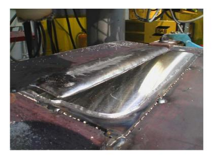
Figure 2.11. Cladding of the second layer after first pass.
