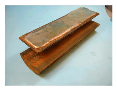
Figure 2.6. Clad, 8 mm thick slice after cutting from ferritic 42CrMo4 steel bar.
