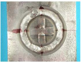
Figure 2.193. Inconel 152 after liquid penetrant testing.
