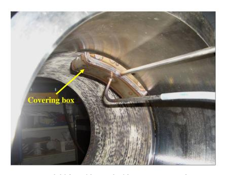
Figure 2.206. Weld root shielding gas covering box.
