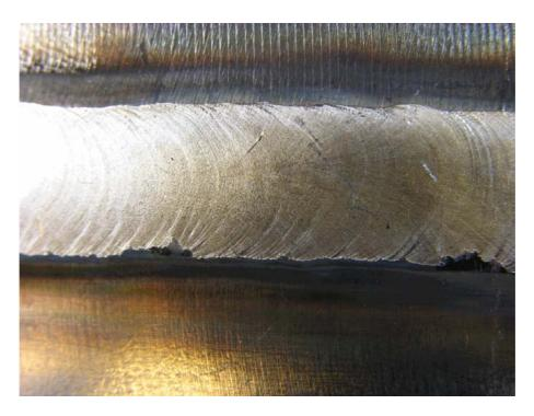
Figure 2.44. Surface of the TV test piece with hot cracks after Varestraint test. Augmented strain was 3%.
