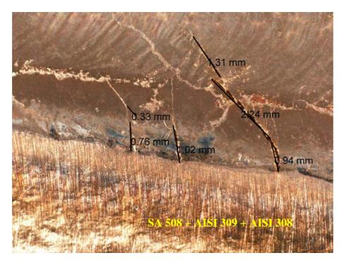
Figure 2.61. Measured crack lengths in mock-up 2 with magnification of 25x and augmented strain of 4%.
