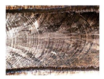
Figure 2.84. Test specimen of Inconel 52MS weld after testing with 4% augmented strain.
