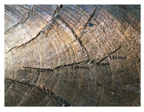
Figure 2.52. Measured crack lengths in mock-up 1 with magnification of 25x and augmented strain of 4%.
