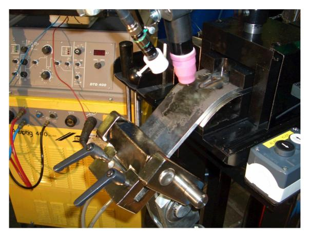
Figure 2.21. Test specimen after bending in Varestraint test.
