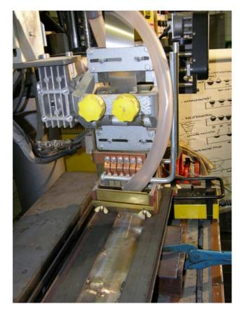
Figure 2.3. Cladding of ferritic 42CrMo4 steel bar by submerged arc welding.
