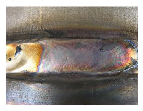
Figure 2.39. Test piece F1 after Varestraint test. Augmented strain was 4%.
