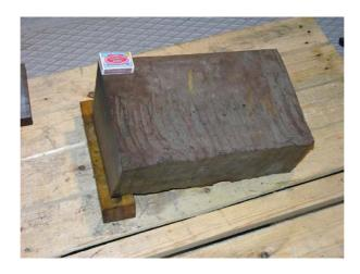
Figure 2.9. Pressure vessel steel (SA 508 Grade 2) piece.
