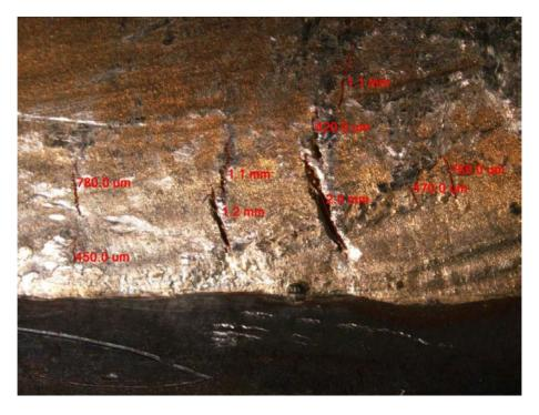
Figure 2.25. Measured crack lengths with magnification of 25x. Augmented strain was 4%.
