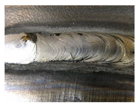
Figure 2.41. Surface of the test piece TV with hot cracks after Varestraint test. Augmented strain was 4%.
