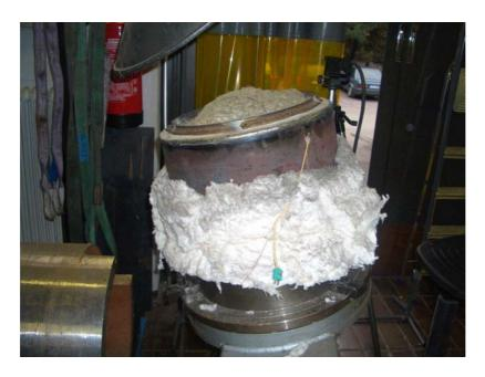
Figure 2.200. Pressure vessel steel pipe fastened to the turning table ready for buttering.
