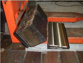
Figure 2.12. Cutting a slice by band saw.
