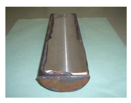
Figure 2.4. Ferritic 42CrMo4 steel bar after cladding and machining.
