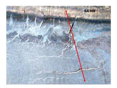
Figure 2.181. Cutting line of cross-section of mock-up 3 sample for microstructural examinations after Varestraint test.
