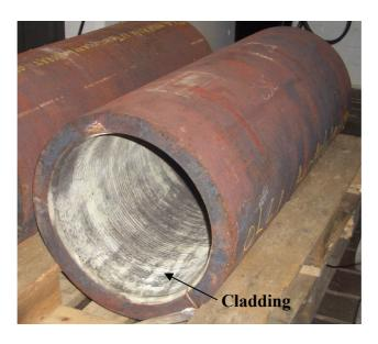
Figure 2.198. Pressure vessel steel pipe with cladding.
