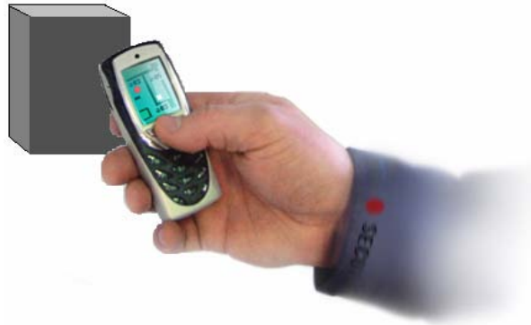
Figure 11. NFC server technology enables using a mobile phone as the user interface for non-UI devices.
