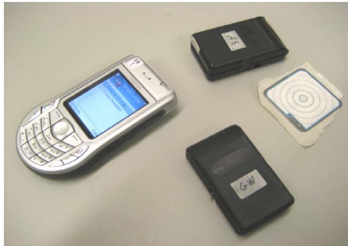
Figure 13. A smartphone with Bluetooth is connected to VTT's Gateway (GW) via Bluetooth. This enables reading (or writing) of data from VTT's NFC/Ambient Server (AS) or from NFC tags to the phone.
