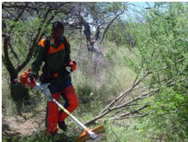
Figure 23. Brush cutter STIHL FS550 at CCF (photo by Arvo Leinonen).
