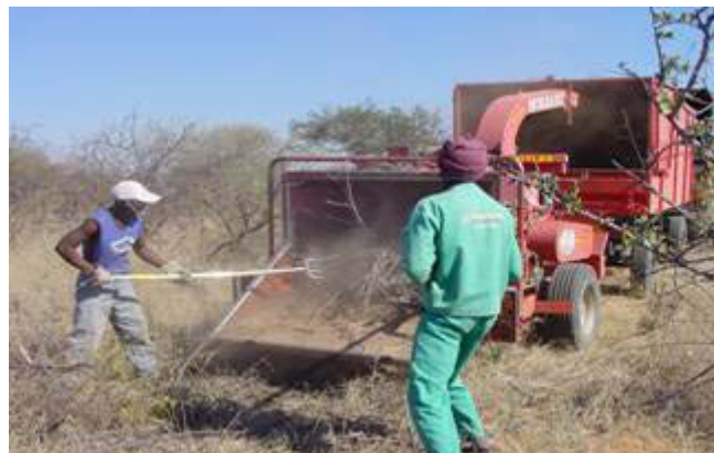
Figure 17. The bush chipping with Morbark Tornado Model 13 drum chipper at CCF in June 2007 (photo by Arvo Leinonen).
