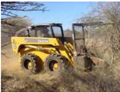
Figure 39. A skid steer (left) equipped with grapple for compiling the bushes (right). Not tested in Namibian conditions.
