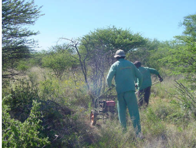
Figure 26. Lawn mower type cutter (photo by Arvo Leinonen).
