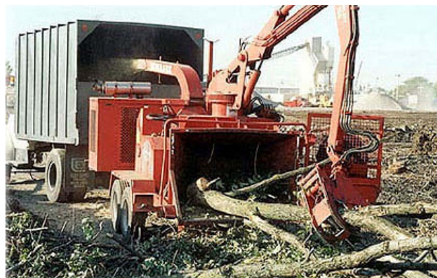
Figure 40. A drum chipper with loader (Morbark Hurricane 18 drum chipper). Not tested in Namibian conditions.
