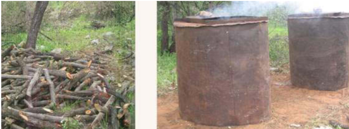
Figure 3. The billets (left) made manually by axes are 'burned' in the kilns (right) at the stand.
