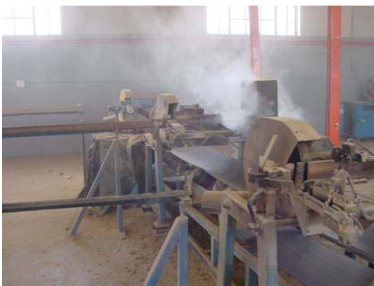
Figure 5. Briquette production line (left) and packaging of briquettes (right) at CCF in Otjiwarongo (photos by Arvo Leinonen).
