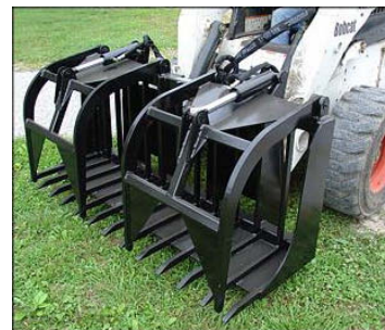
Figure 39. A skid steer (left) equipped with grapple for compiling the bushes (right). Not tested in Namibian conditions.
