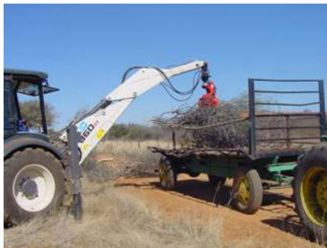
Figure 32. The bushes are loaded to the trailer by Nisula harvester head (photo by Arvo Leinonen).
