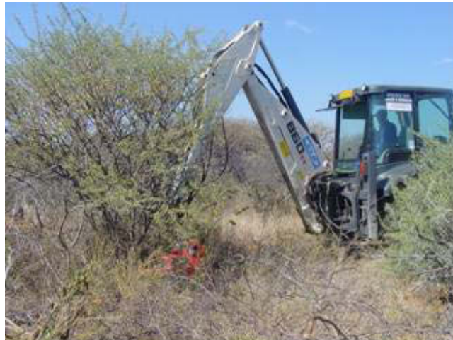
Figure 29. Nisula harvester head at work (photo by Arvo Leinonen).
