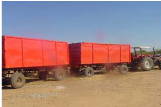
Figure 20. Tractor unit for bush chips road transport at CCF in June 2007 (photo by Arvo Leinonen).
