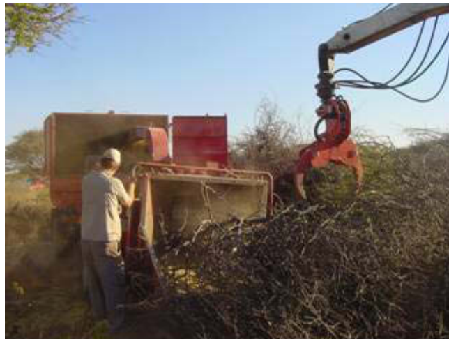
Figure 36. Feeding of the bushes to the chipper by Nisula harvester head (photo by Arvo Leinonen).
