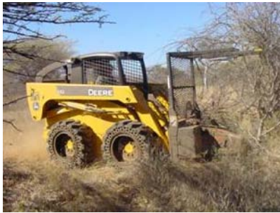
Figure 38. A skid steer (left )equipped with a rotary saw for felling (right). This machine is tested in Namibian conditions (photos by Arvo Leinonen).
