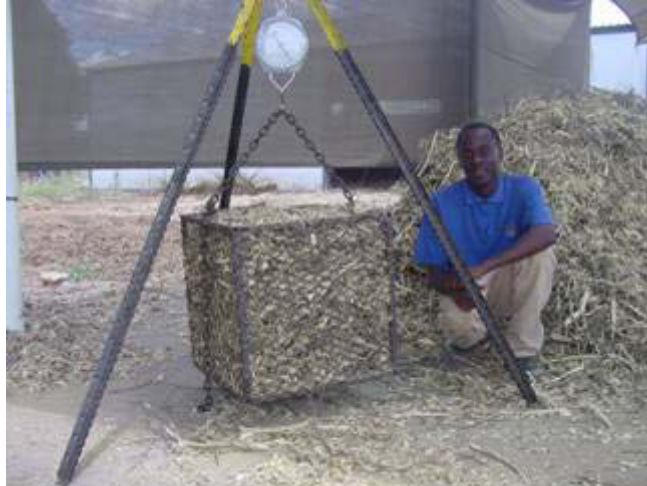
Figure 37. Measuring the wood chip loose density at CCF briquette factory in Otjiwarongo (photo by Arvo Leinonen).
