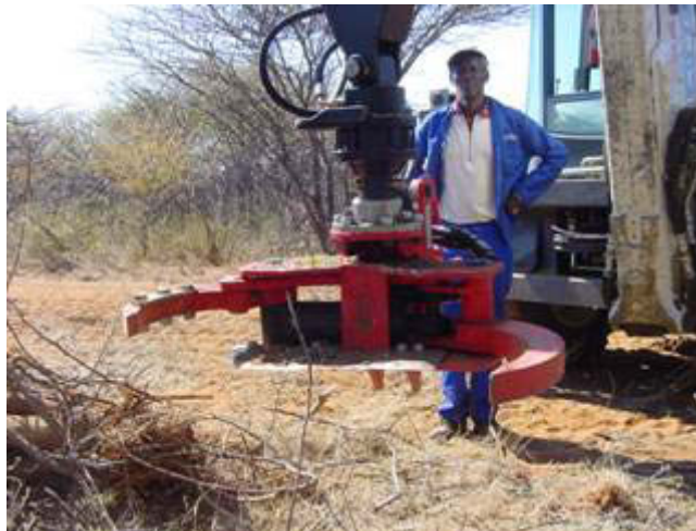
Figure 27. Nisula harvester head mounted on the boom in Terex backhoe loader. The pressing arms and cutting blade can be seen in the picture (photo by Arvo Leinonen).
