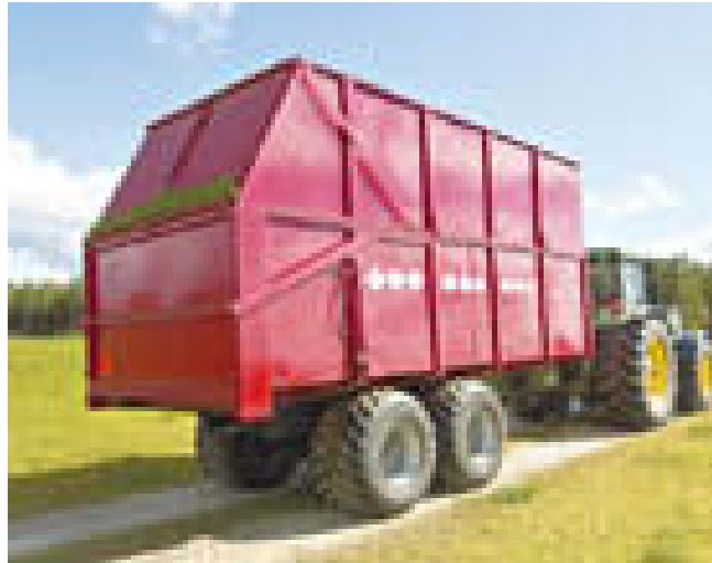
Figure 41. Tractor trailer for road transport of wood chips (Junkkari 18 from Finland). Not tested in Namibian conditions.
