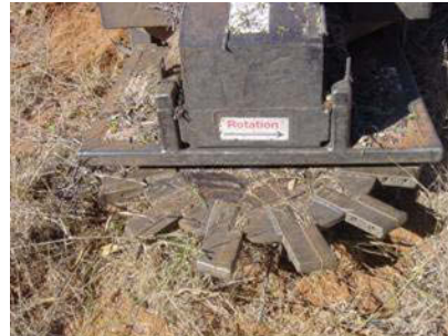
Figure 38. A skid steer (left )equipped with a rotary saw for felling (right). This machine is tested in Namibian conditions (photos by Arvo Leinonen).
