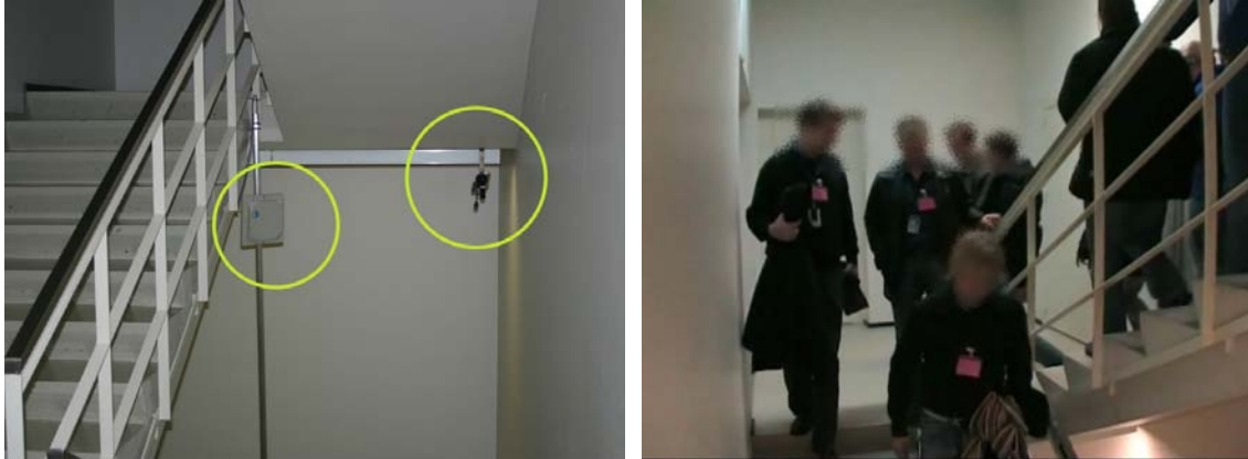
Figure 8. Left side: monitoring equipments between floor levels (RFID-antenna and DV-camera). Right side: snapshot of the DV-camera during the evacuation exercise.
