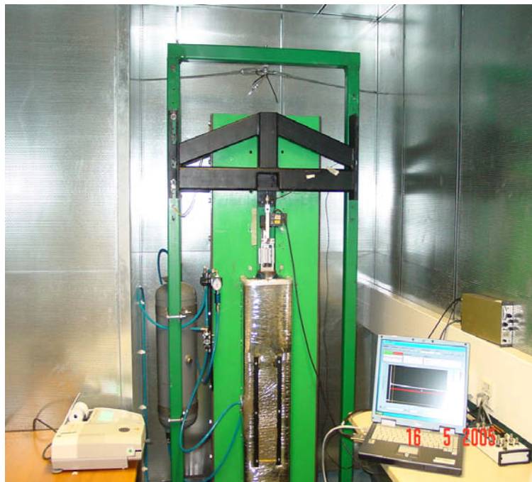
Figure 100. Fast tensile test rig IMPACT.
