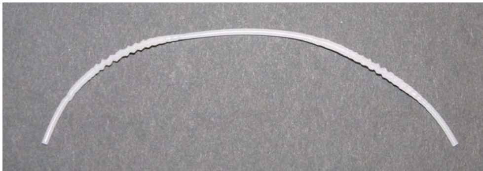
Figure 32. Distortions in the material after capillary rheometer experiment.
