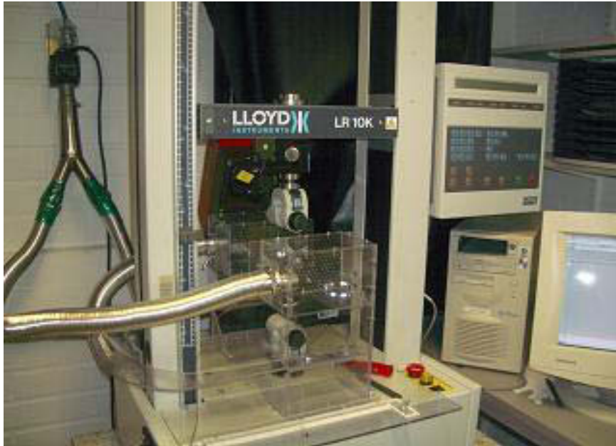
Figure 108. Equipment used in drying stress measurements.
