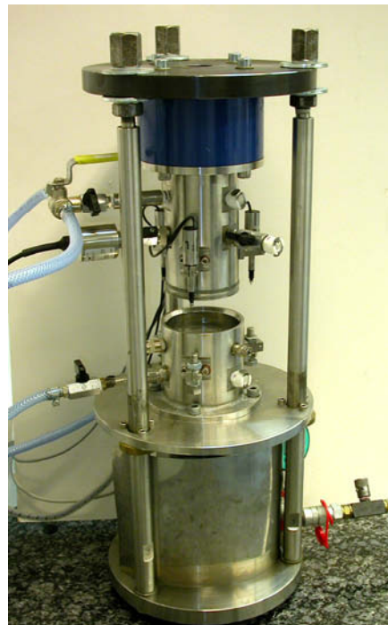
Figure 83. Permeability cell used to measure the flow resistance of card board samples under compression.
