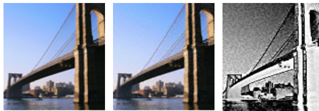
Figure 2.2. The principle of digital watermark. From left: original image, image with digital watermark and digital watermark i.e. modified pixels. (Image source: Digimarc, www.digimarc.com )
