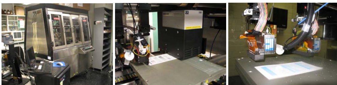
Figure 4.5. Inkjet research environment at VTT. From left: XY-table for moving the substrate (right, XY-MDS) and control unit for the printheads (Apollo II), online UV-curing and industrial printheads for 4-colour printing (two printheads shown).
