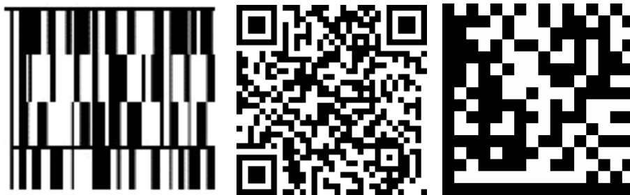
Figure 2.1. Two-dimensional bar codes: from left Code 49, QR Code and Data Matrix.
