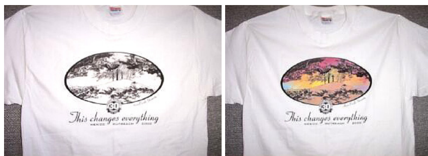
Figure 4.7. T-shirt printed with photochromic ink indoors (left) and outdoors (right). (Image source: Chromatic Technologies International, www.ctiinks.com )
