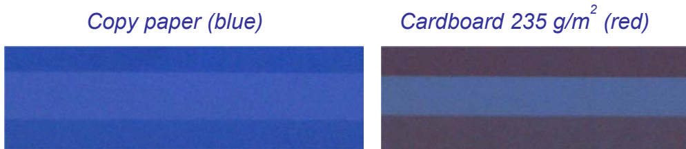
Figure 4.10. Photographing with black light lamp radiation. The UVA value was 4500 \text{ mW/m}^2 . It can be seen in the middle of the pictures that Black Light Lamp has blued the substrates.
