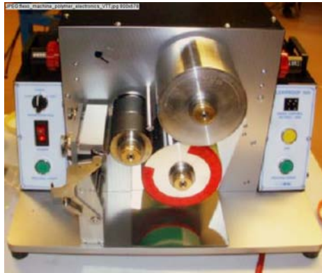
Figure 4.3. Flexiproof-100 printer (RK Print-Coat Instruments Ltd) that was used in printing the thermochromic samples.
