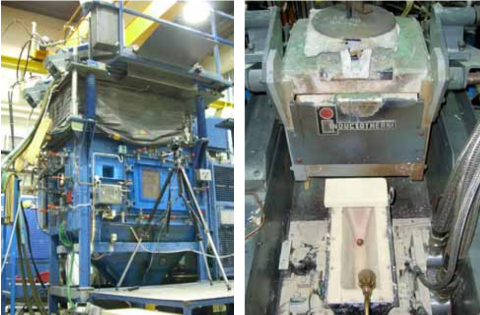
Figure 20.2.2. Photographs of the HECLA facility and its induction furnace.
