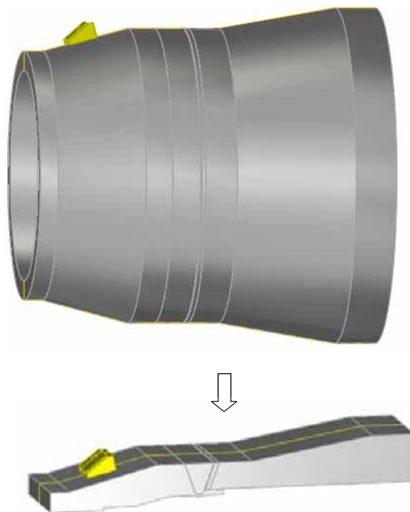
Figure 25.2.3. The original tubular nozzle geometry and the simplification to planar geometry model. In the planar geometry the weld design details can be seen.
