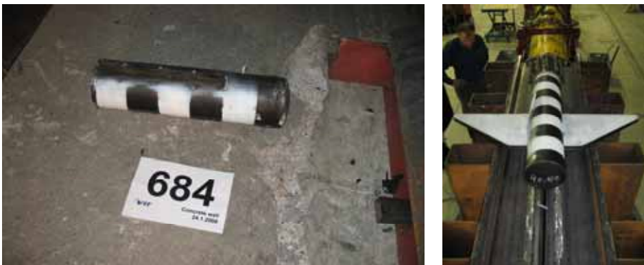
Figure 29.1.3. The rigid steel pipe missile with a diameter of 150 mm (left) and an aeroplane model with wings (right).
