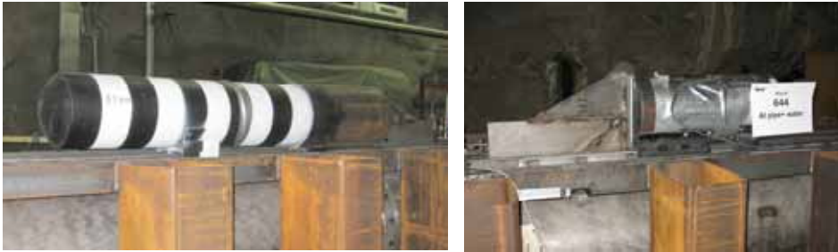
Figure 29.1.2. Dry (empty) aluminium (Al) pipe missile and wet (water filled) missile.
