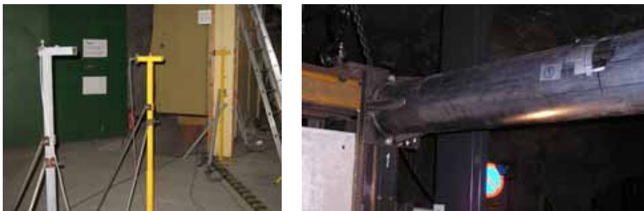
Figure 29.1.6. The laser sensors (left) and a strain gauge on the back pipe (right).
