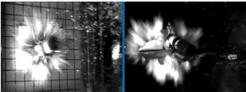
Figure 29.1.17. Typical liquid splash pattern from a cylindrical (left) and a prototypical 3D missile (right).
