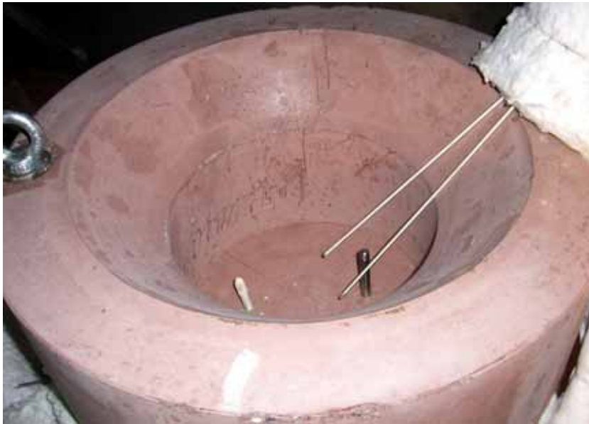
Figure 20.2.4. HECLA-3 concrete crucible before the experiment.
