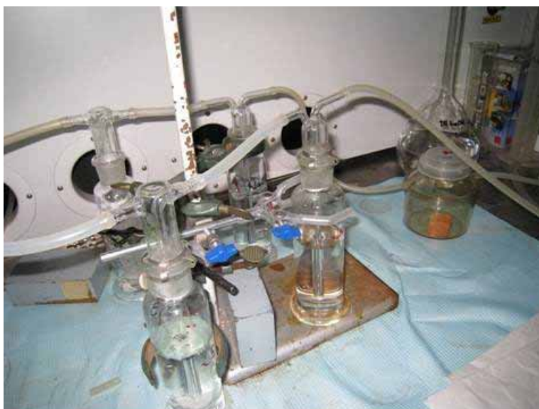
Figure 18.1.3. Traps to collect different forms of iodine.
