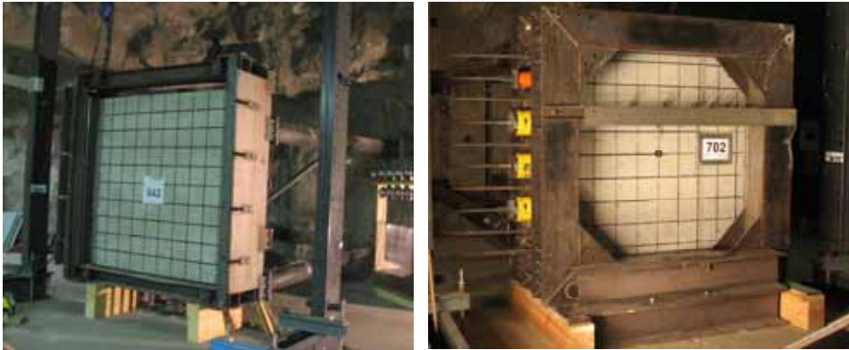
Figure 29.1.4. One way support system and test slab in soft missile test (left). Pre-stressed test slab with a thickness of 0.25 m and support system 2 in hard missile test (right).
