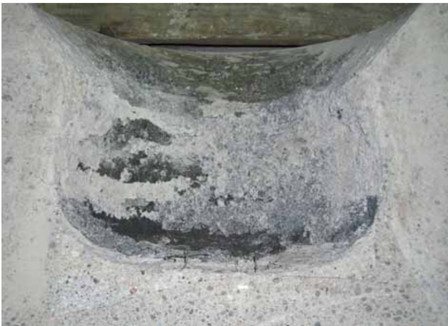
Figure 20.2.8. The HECLA-2 concrete crucible after splitting and removing the metal ingot.
