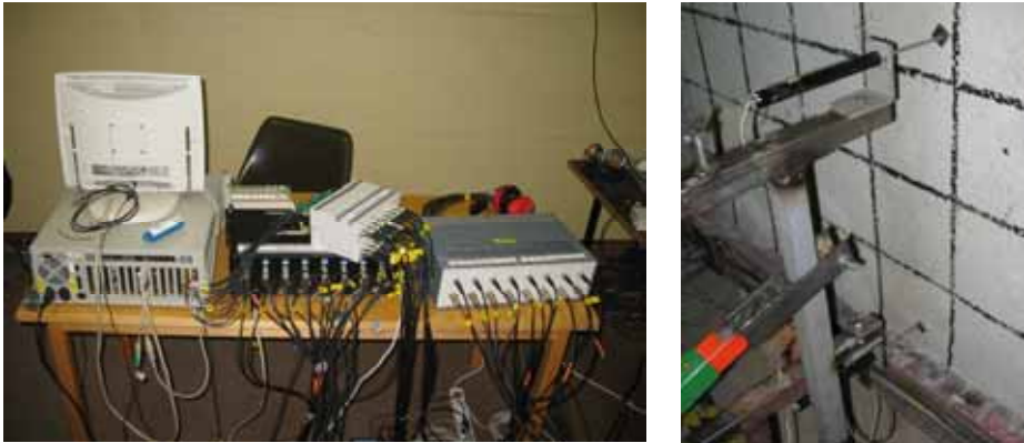
Figure 29.1.5. Measuring data collection device (left) and deflection transducers in front of the slab (right).
