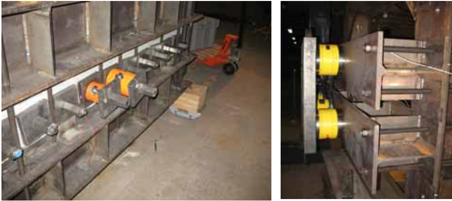
Figure 29.1.7. The force transducers of Dyvidag bars (left) and the force transducers behind the force plate (right).
