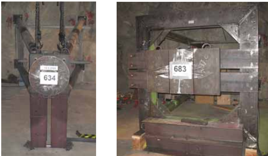
Figure 29.1.1. The second model (left) and third model of force plate construction.
