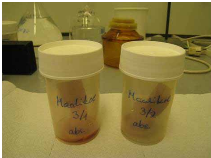
Figure 18.1.2. The painted blocks adsorbed gaseous iodine on the surface from the air.
