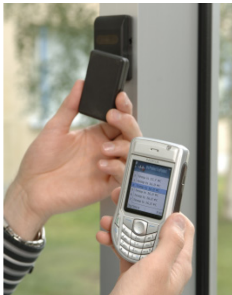
Figure 86. NFC enabled temperature sensor is being read by touching with NFC-Bluetooth Gateway. Temperature readings are show on the display of the mobile phone.
