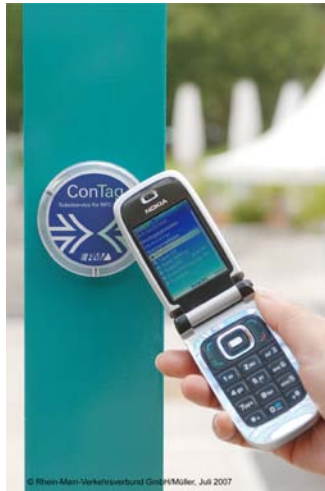
Figure 38. ConTag attached to a station pole.
