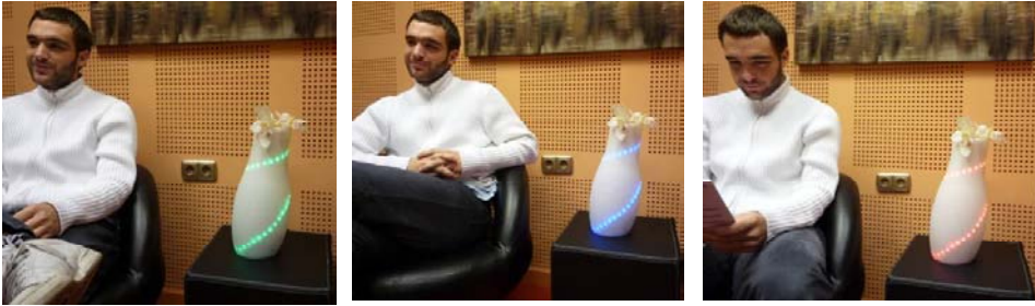
Figure 96. Table lamps showing three different temperature statuses related to the desired temperature: green for optimal temperature achieved, blue for colder temperatures and red for warmer temperatures.
