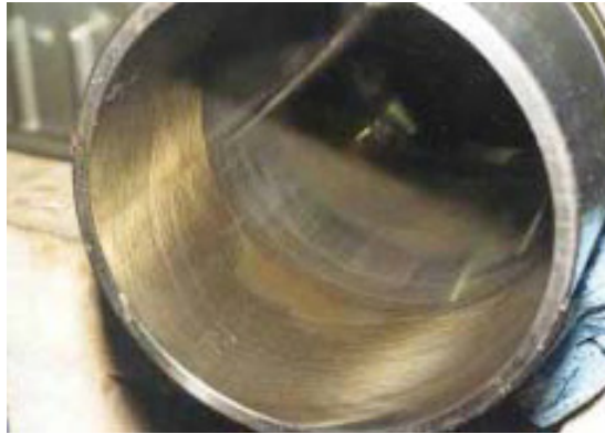
Figure 5. Gold-coloured siloxane layer on the inner surfaces of a cylinder (Environmental Agency 2002).
