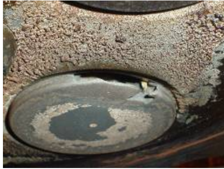
Figure 13. Damage on inlet valve at cylinder head.
