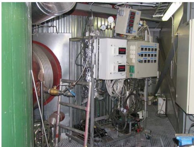
Figure 6. The slip stream catalyst testing facility connected to the raw gas line between the Novel gasifier and the main stream reformer.
