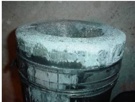
Figure 14. Damage on piston.
