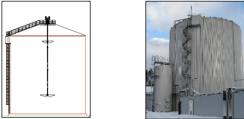
Figure 6. Layout of the Full-Scale Reactor.
