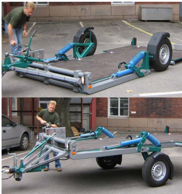
Figure 3. The prototype trailer in its highest and lowest positions.
