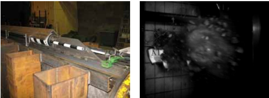
Figure 7. Hard missile with a tail (left). Concrete wall and dust after perforation (right).
