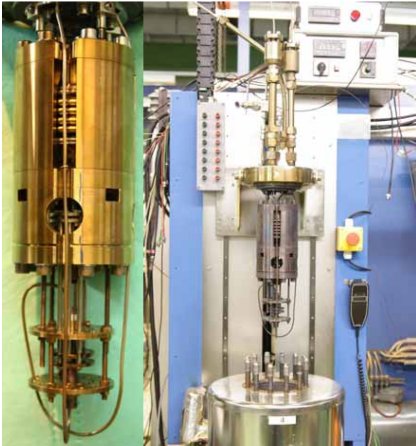
Figure 4. FABELLO unit before and after three months in 300°C pressurised water.
