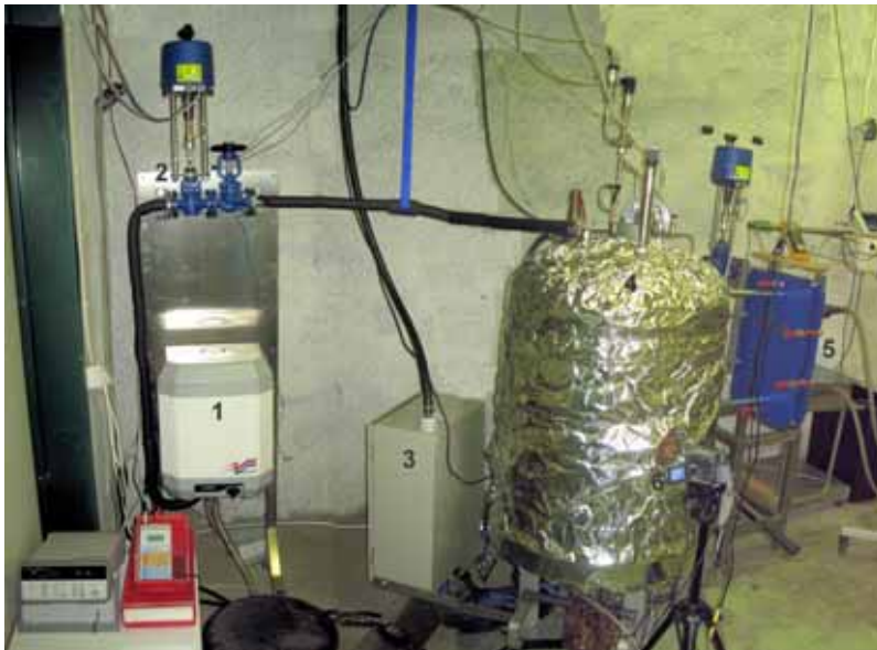
Figure 1. An overview of the COOLOCE test facility. The components are 1) feed water pre-heater, 2) feed water control valve, 3) connection box for the electrical heaters 4), pressure vessel, 5) condenser and scale for measuring condensate mass flow, 6) video monitoring and 7) pressure gauges.
