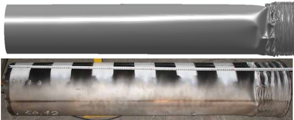
Figure 12. The deformed missile of test FP8 in the FE simulation and in the real test.
