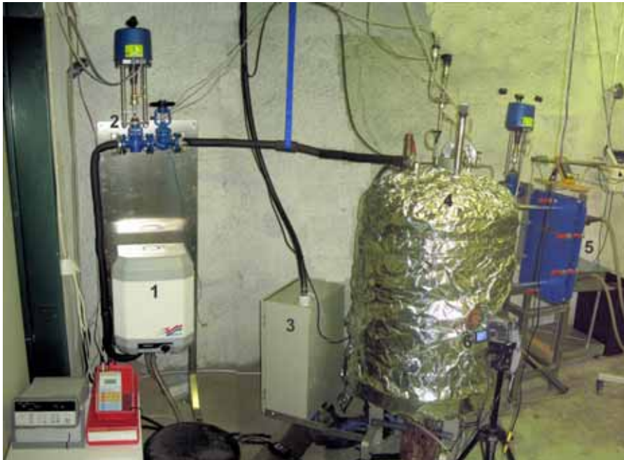
Figure 2. An overview of the COOLOCE test facility. The components are 1) feed water pre-heater, 2) feed water control valve, 3) connection box for the electrical heaters 4), pressure vessel, 5) condenser and scale for measuring condensate mass flow, 6) video monitoring and 7) pressure gauges.
