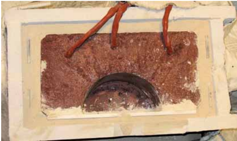
Figure 3. VULCANO VB-U7 concrete crucible before the experiment.
