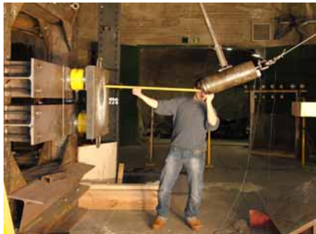
Figure 4. Schematic drawing of the heavy impact hammer and picture of a test performance.
