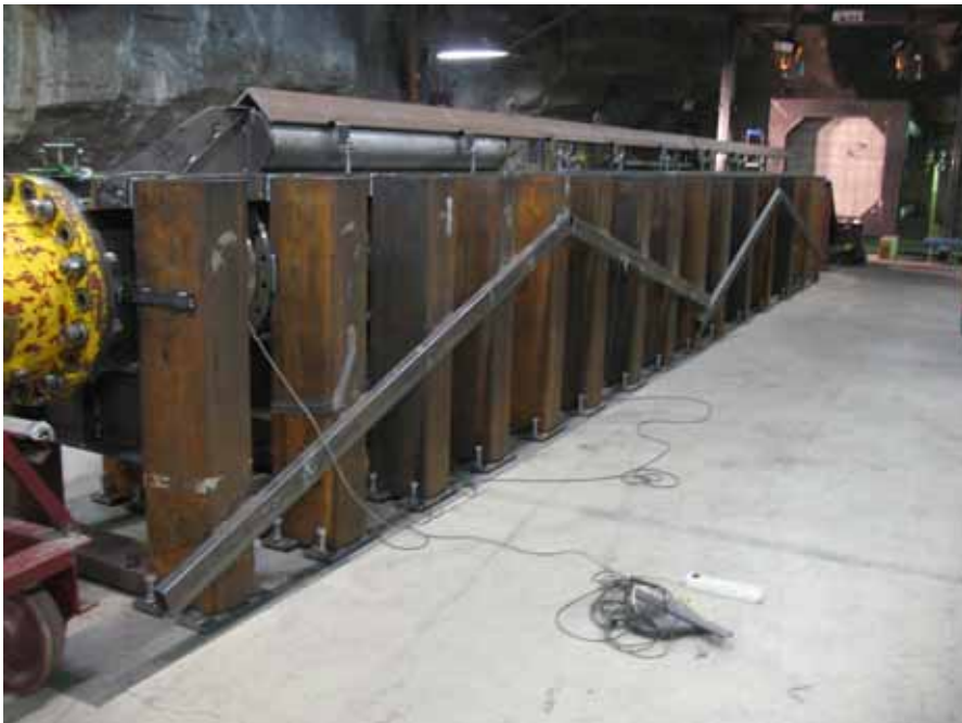
Figure 1. Modified impact apparatus in 2011.
