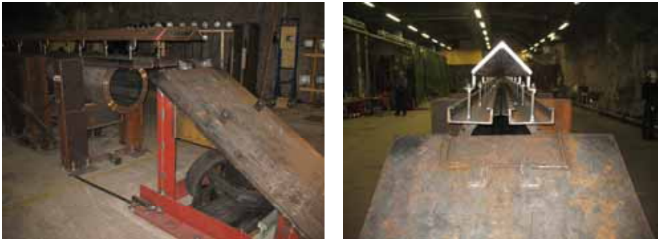
Figure 2. The corner profile installed above the acceleration tube.
