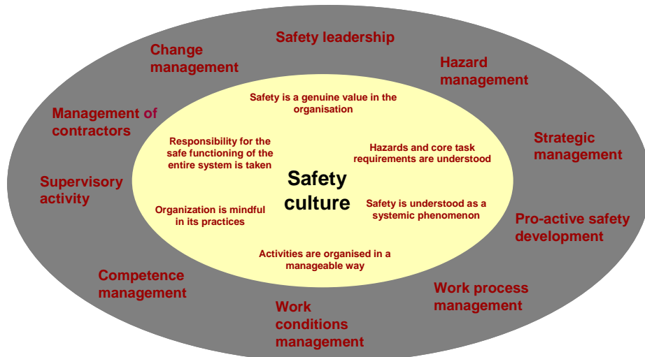
Figure 1. This figure presents the basic elements of the DISC-model; the criteria for good safety culture (inner circle) and the organisational functions (outer circle) which are necessary for developing good safety culture in the organisation.
