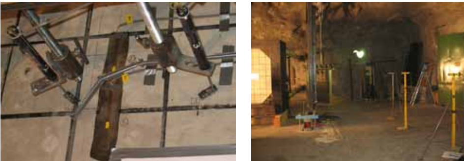
Figure 6. Strain gauges glued on the front surface (left) and laser sensors (right).
