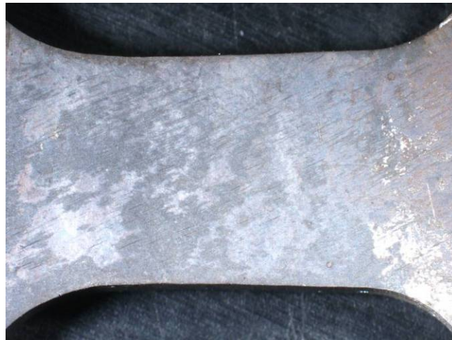
Figure 29. Alloy 182 test specimen surface after a DDC test at 1000°C up to 4% of plastic strain. No indications of DDC cracks are visible.
