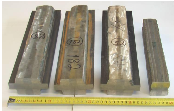
Figure 59. Four welded Ni-base alloy blocks: from the left Alloy 82, 182, 52 and 152.
