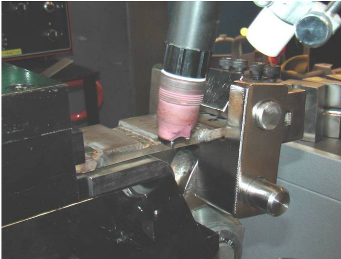
Figure 107. Trans-Varestraint testing of the test sample with almost filled weld metal. The Varestraint testing parameters are shown as an insert in the figure.
