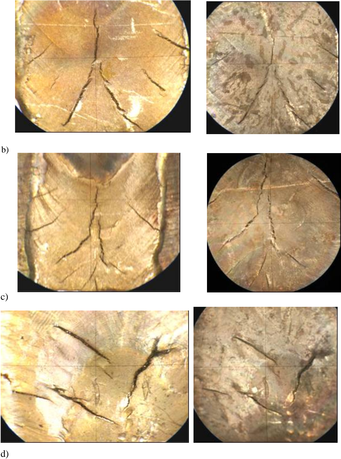
Figure 85. Pure alloy welds after hot cracking in Vareststraint test and after 750 h testing in doped steam. a) Alloy 182 (specimen No. 35), b) Alloy 82 (specimen No. 36), Alloy 152 (specimen No. 37), and d) Alloy 52 (specimen No. 38).
