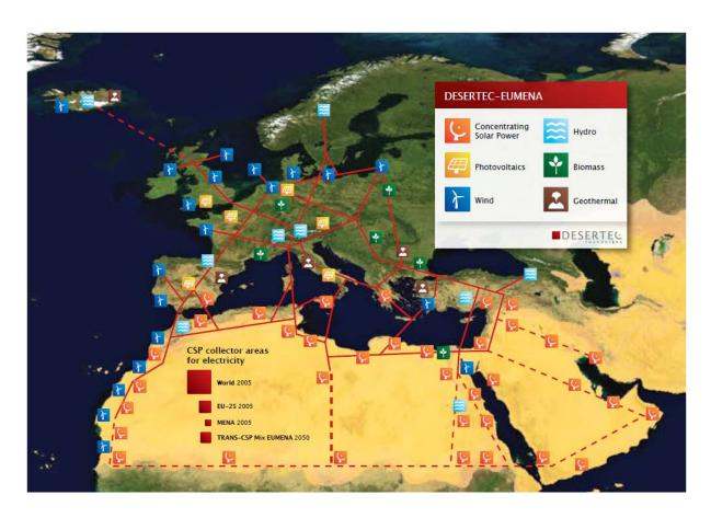
Figure 36. Concept of a "EUMENA Supergrid" based on HVDC power transmission as "Electricity Highways" to complement the conventional AC electricity grid, as developed by TREC in 2003. The symbols for power sources and lines are only sketching typical locations. Reprinted from Desertec Foundation 2009.
