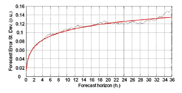
Figure 38. Normalized standard deviation of wind power forecast error for 12 GW installed capacity versus forecast horizon. (Reprinted from Gibescu et al. 2009)
