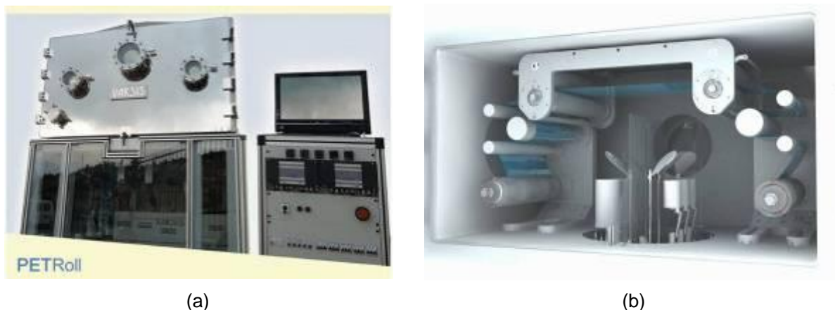
Figure 5. The pictures of the vacuum web coater: (a) from outside and (b) from inside.
