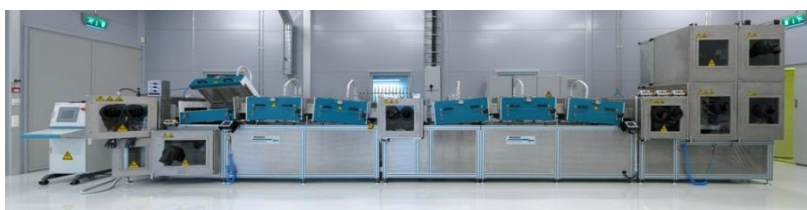
Figure 7. R2R Inert atmosphere printing pilot line with gravure and rotary screen printing and lamination located in VTT, Oulu.
