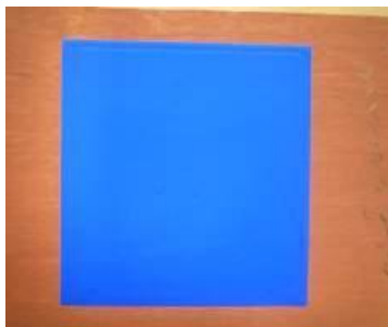
Figure 21. Membrane (PVdF G1 with 2% of Fillers CEA ) directly printed onto negative graphite based electrode
