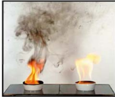
Figure 5.5. Diesel fuels burning in open beakers. Conventional diesel fuel on the left, paraffinic diesel fuel on the right. (ASFE 2006)
