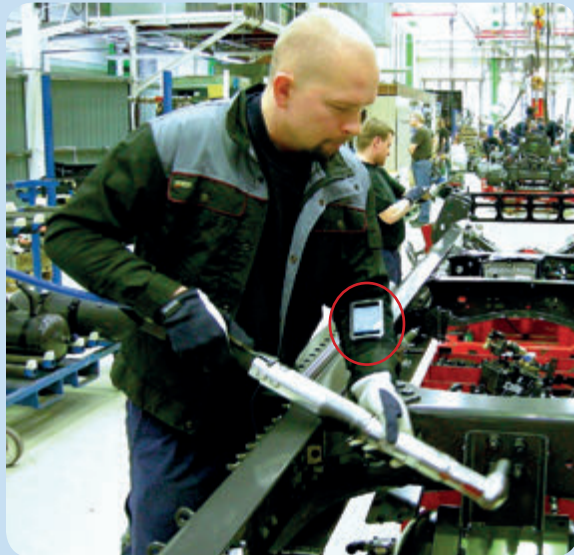
FIGURE 2.3. Mobile operator support for Volvo truck manufacturing (photo: Johan Stahre, Chalmers University)
