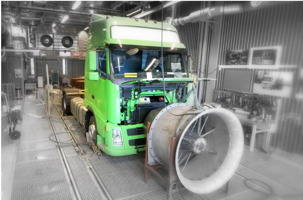
Heavy-duty vehicle test facility at VTT enables simulation of driving in closely-controlled laboratory environment for maximum accuracy and repeatability.
