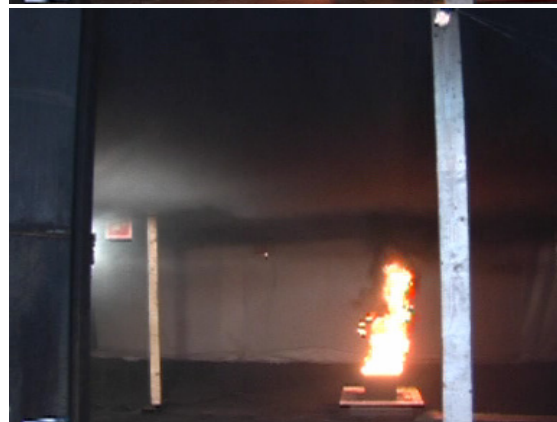
Figure 21. Camera 2 view inside the test compartment. The red exit signs are at the height of 2 m at the level of the line shown in uppermost picture.
