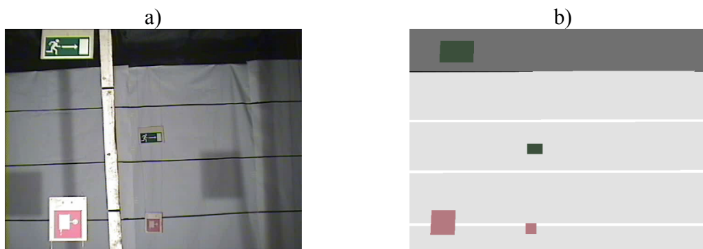
Figure 9. View inside the test compartment: a) photograph and b) the FDS model. The RGB-values of the objects and surfaces in FDS model were close to the RGB values of photographs taken before the experiments. The FDS view was built-up placing the camera to the same position as it was in the experiments and zoomed closer to the objects.
