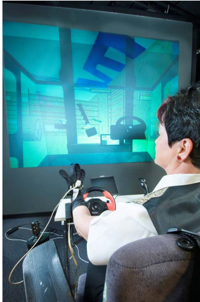
Figure 26. Example of designing cabin layout in VR with data glove.
