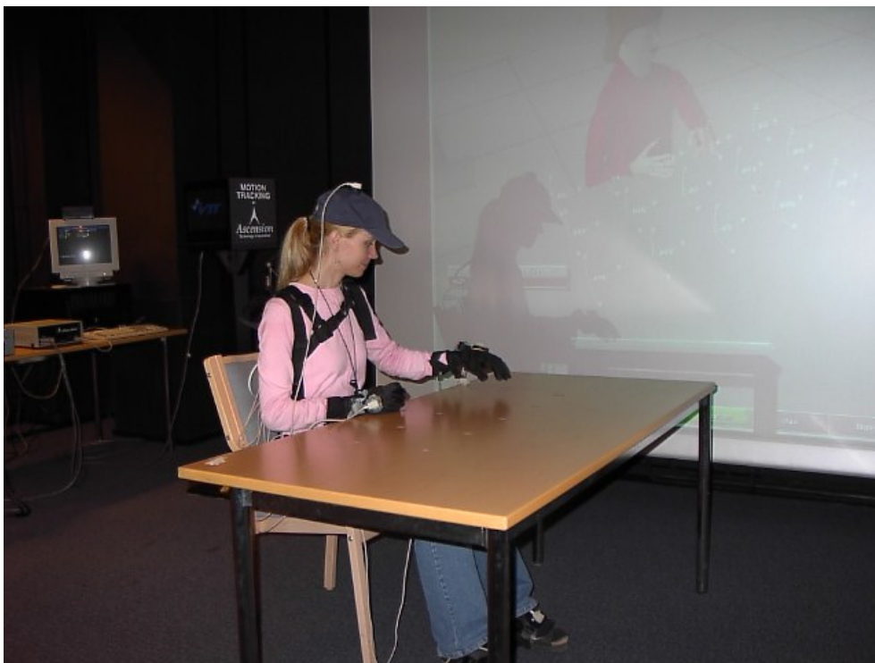
Figure 1. A testing system and a test person's location to table having on surface the matrix points of 2 x 2 centimetres in order to record motions by using a magnetic based wide range human motion capture system.
