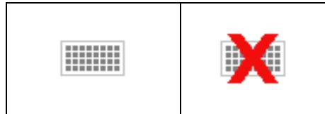
*Figure 7. Icons in N810 status bar indicate whether keyboard service is enabled and available or whether it is disabled or unavailable.*
