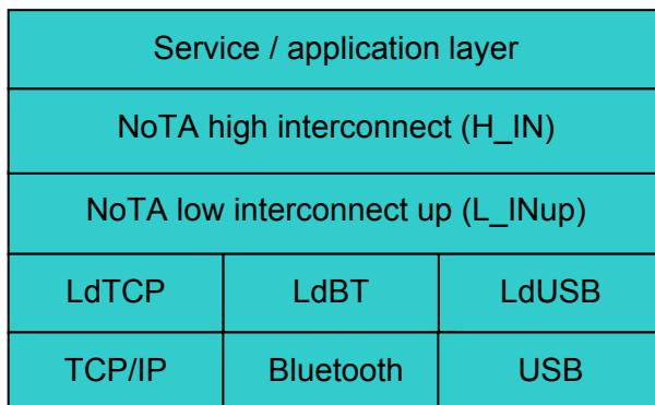
*Figure 2. NoTA protocol stack with few transport alternatives.*
