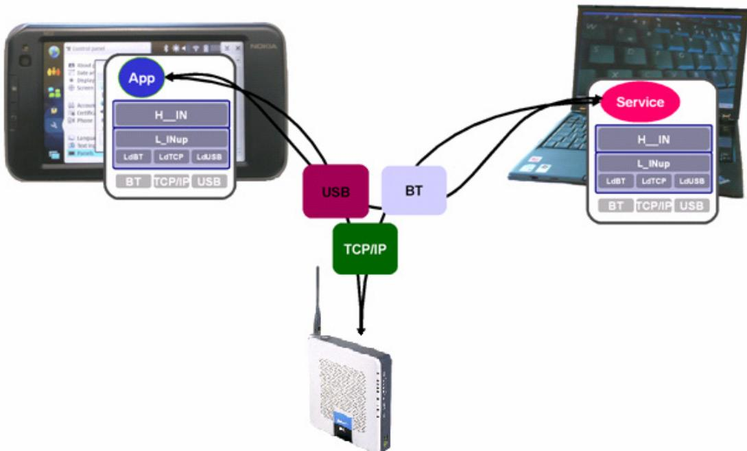
Figure 1. NoTA Keyboard service – components and example deployment to N810 internet tablet and Linux laptop.
