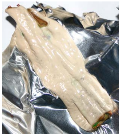
Figure 30. Melted MMJ sample on Al-foil after a test where T_{\max} near the sample was 240 °C.
