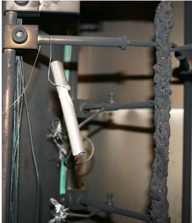
Figure 32. Charred MMJ cable sample after experiment MMJ2. The white reference cable sample to the left is slightly deformed only at point of suspension.
