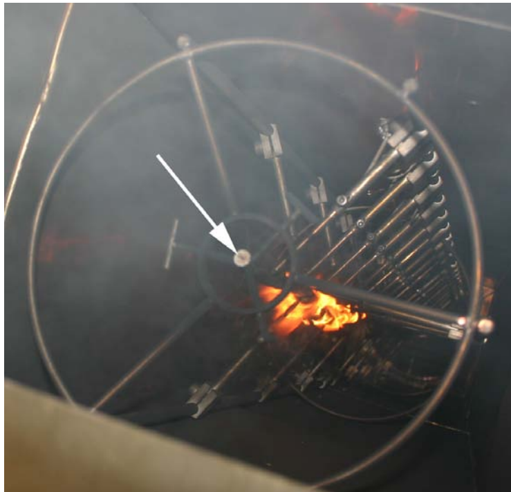
Figure 31. Flame spread on a MMJ cable sample in experiment MMJ1, photograph from above through the smoke outlet. The upper end of the sample is indicated with an arrow.
