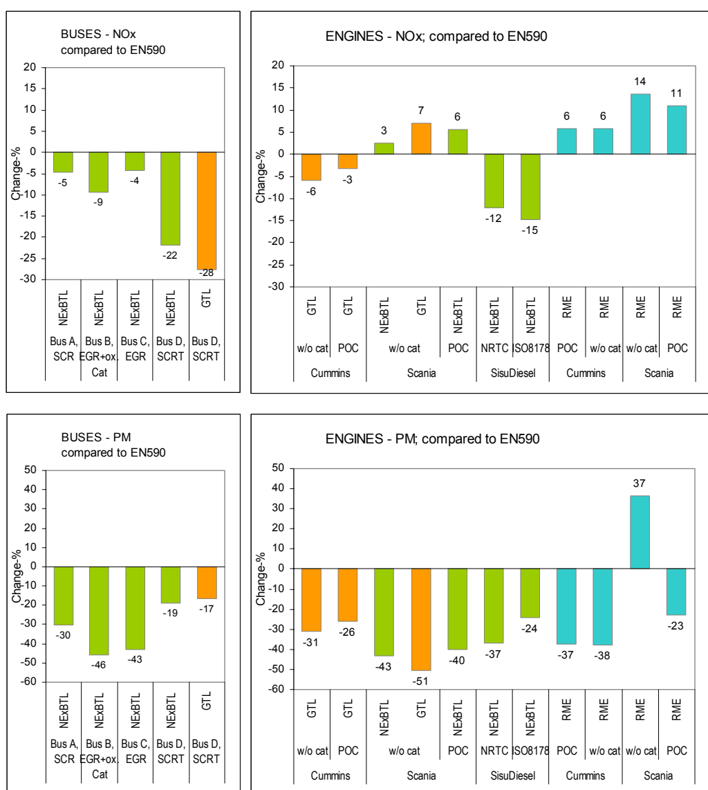
Figure 73. The difference in NO x and PM emissions when NExBTL, GTL and RME are compared to the EN590 fuel.
