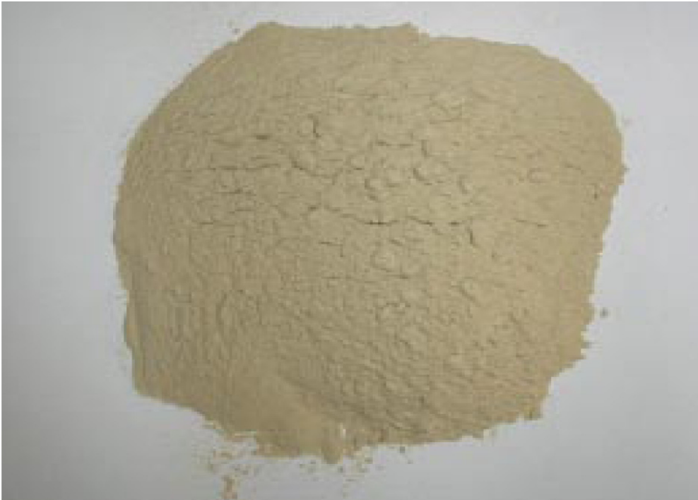
Figure 2-6. Milos non-activated high-grade bentonite Deponit CA-N /Karnland et al. 2006/.
