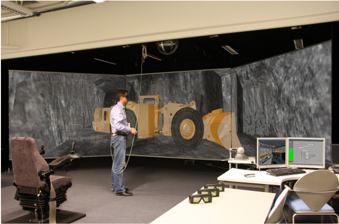
Figure 3. Virtual Environment system for Cabin design used onsite at VTT.
