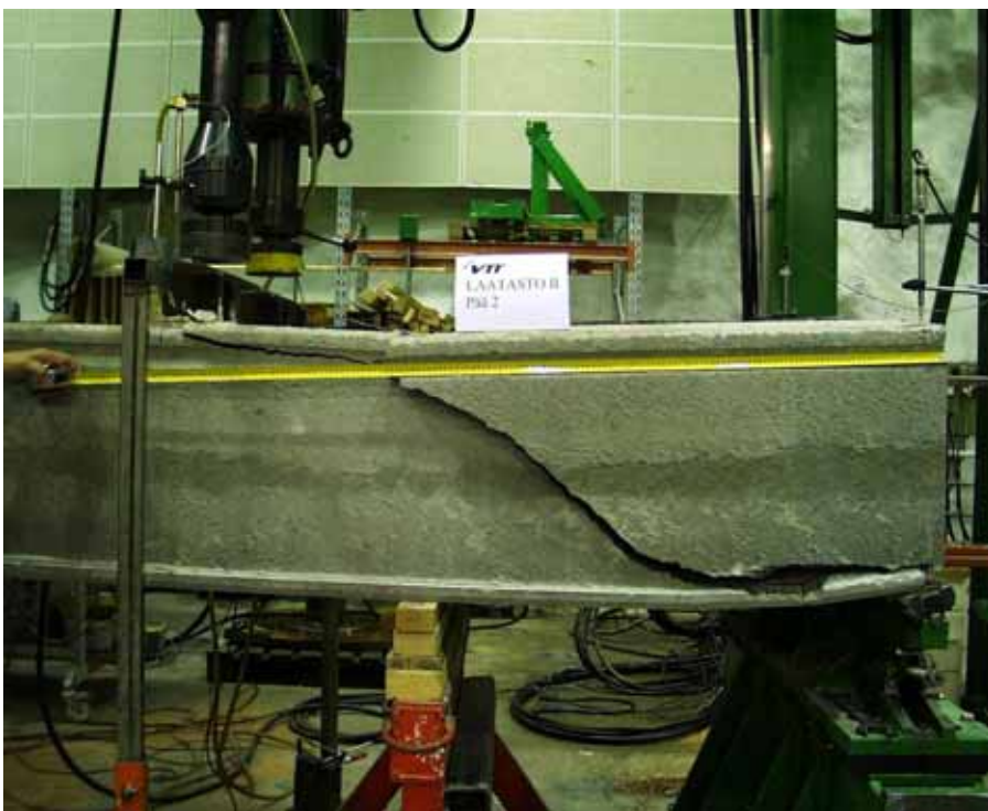
Fig. 2. Failure mode in reference test R2.
