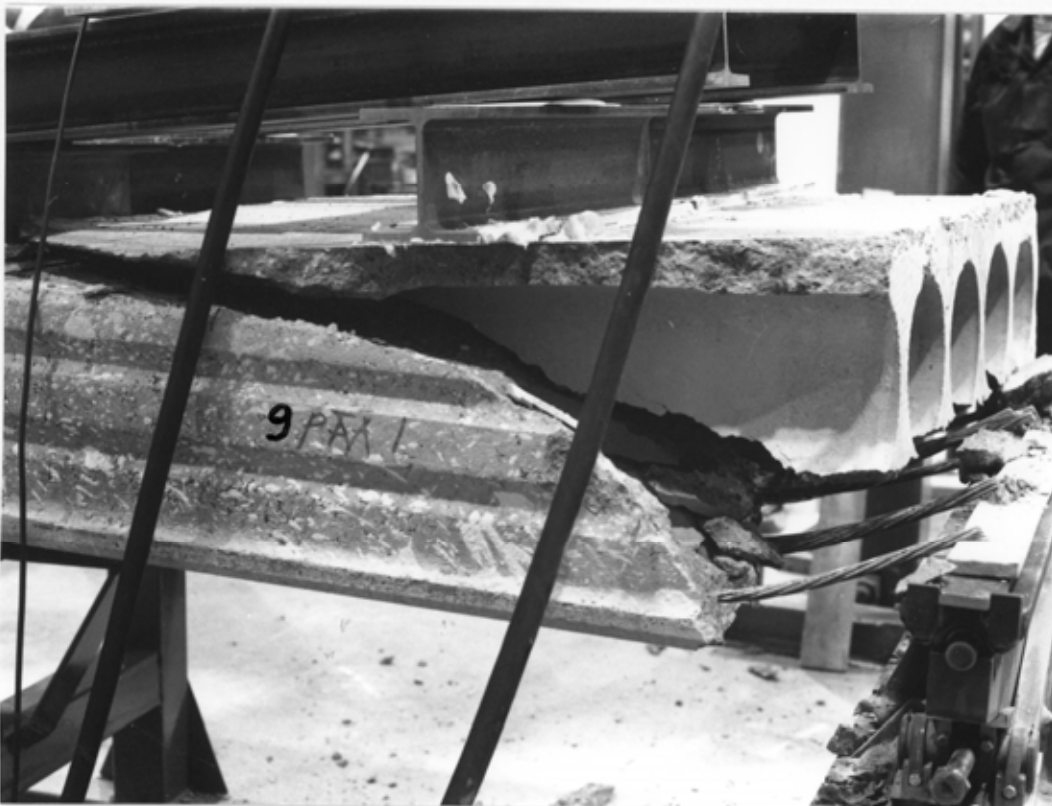
Fig. 25. Reference test R1. Failure pattern.
