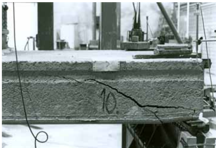
Fig. 21. Failure pattern of slab unit 10 in reference test.
