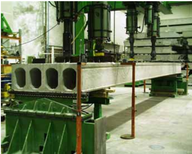
Fig. 27. Overview on arrangements in reference tests. The actuators in the rear were not used.
