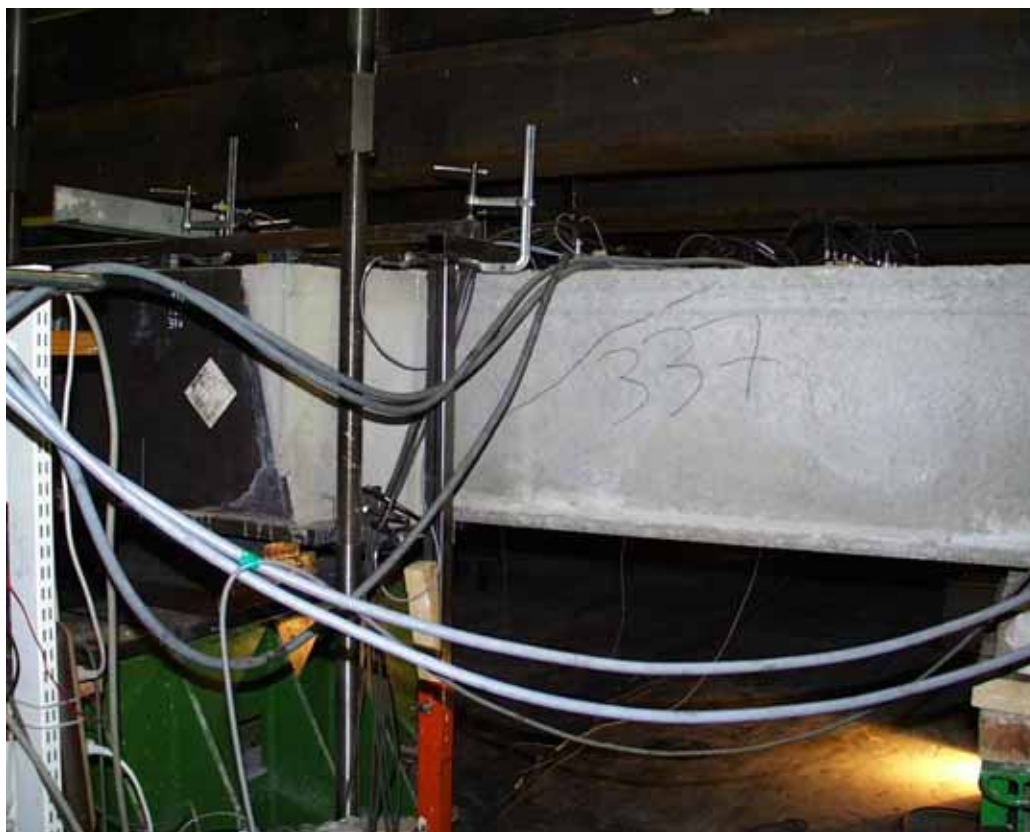
Fig. 17. Shear crack in slab 1 at P_a = 337 kN.
