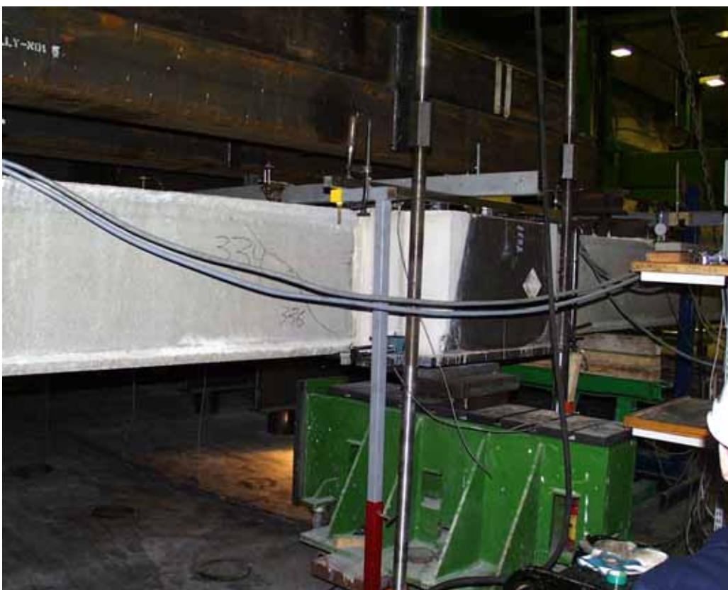
Fig. 16. Shear cracks in slab 7 at P_a = 336 kN.
