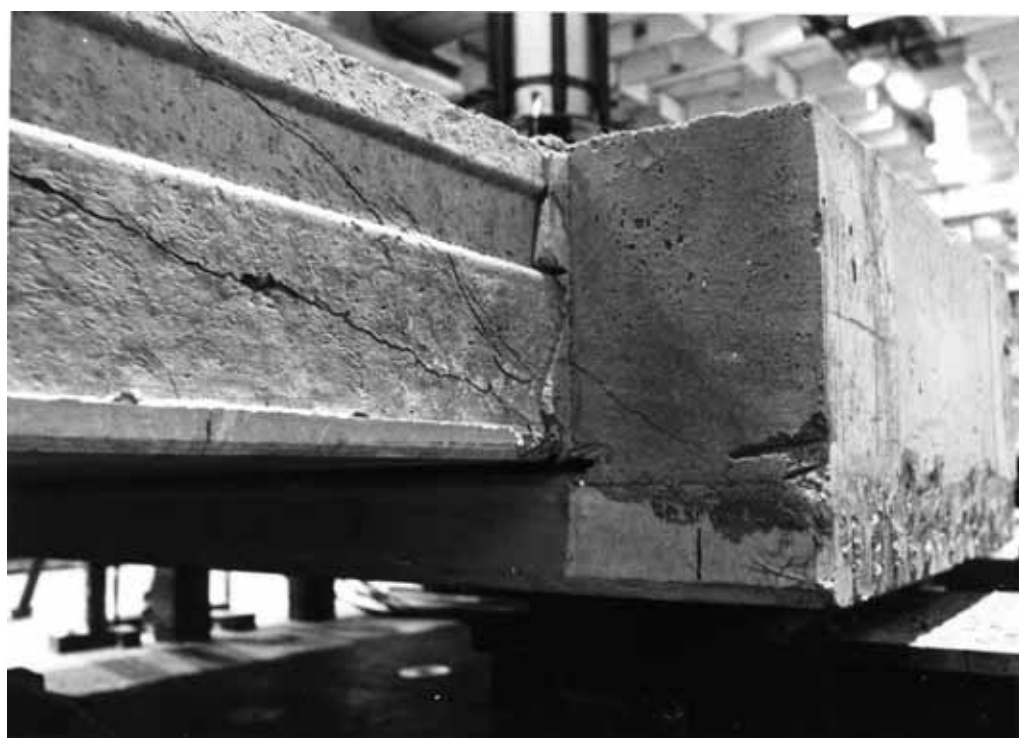
Fig. 19. Failure of slab 5.
