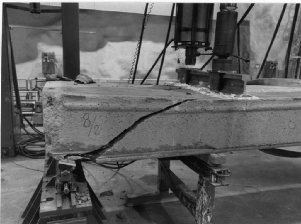
Fig. 13. Failure pattern of slab unit no 8 in reference test.
