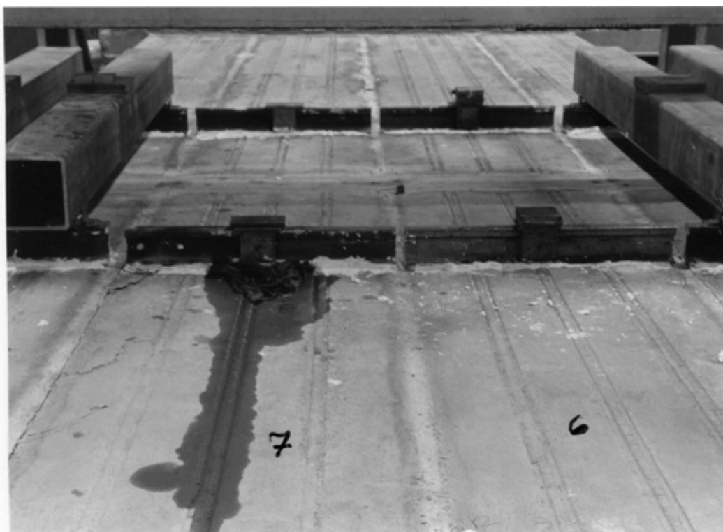
Fig. 10. Failure at stage 2 seen from above after removal of loading equipment.
