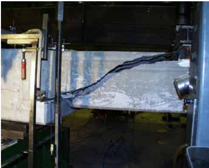
Fig. 13. Failure of slab 8.
