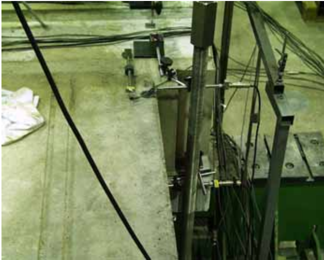
Fig. 7. Transducers measuring differential horizontal displacement at one end of the middle beam.
