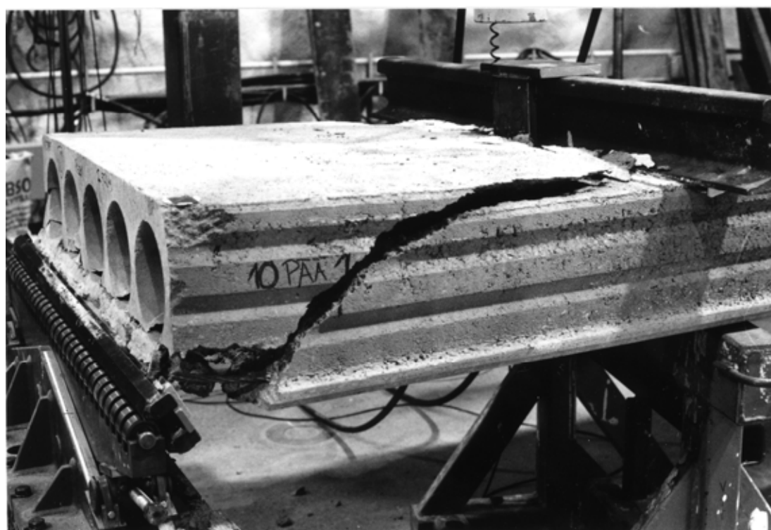
Fig. 16. The failure of the end 1 of the slab unit no 10 in the reference loading test.
