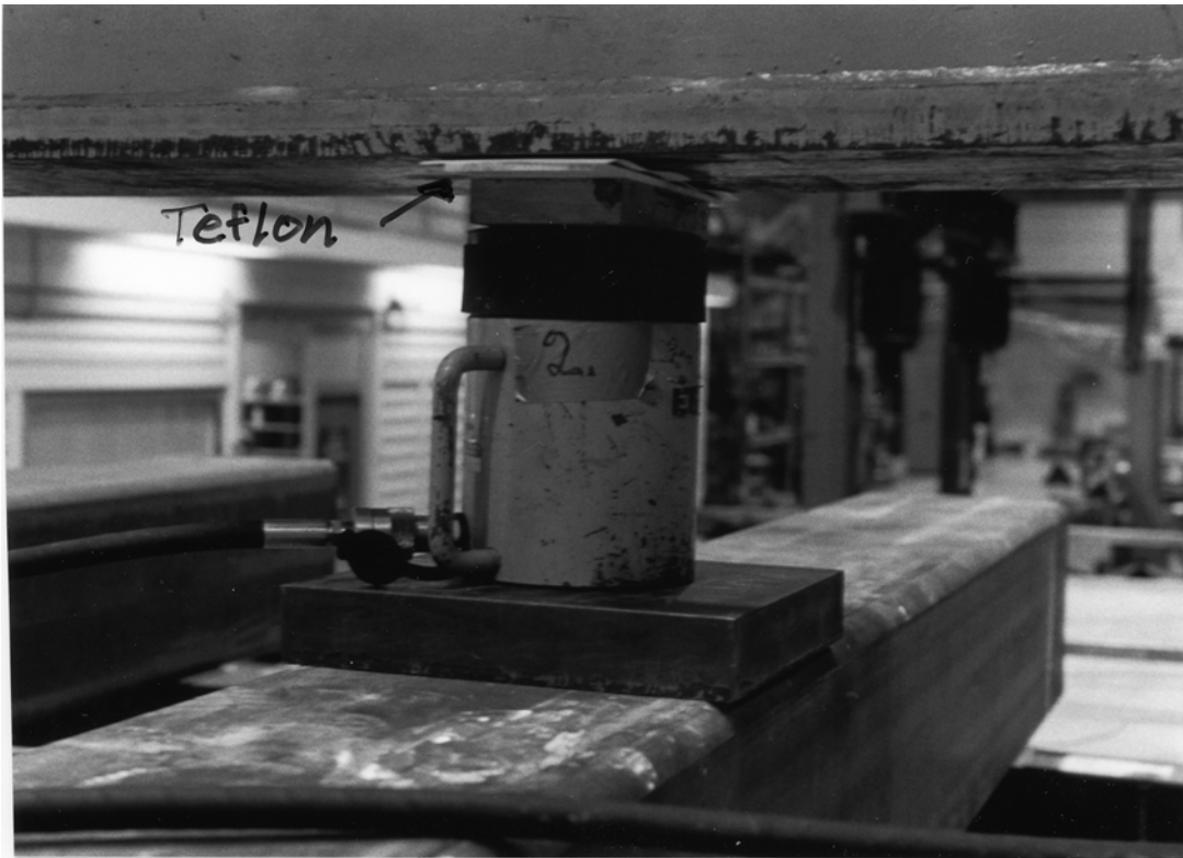
Fig. 3. Hydraulic actuator between the loading frame and a tertiary spreader beam. Note the teflon sheets.
