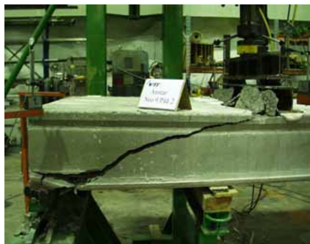
Fig. 48. Reference test R2. Northern side of slab after failure.
