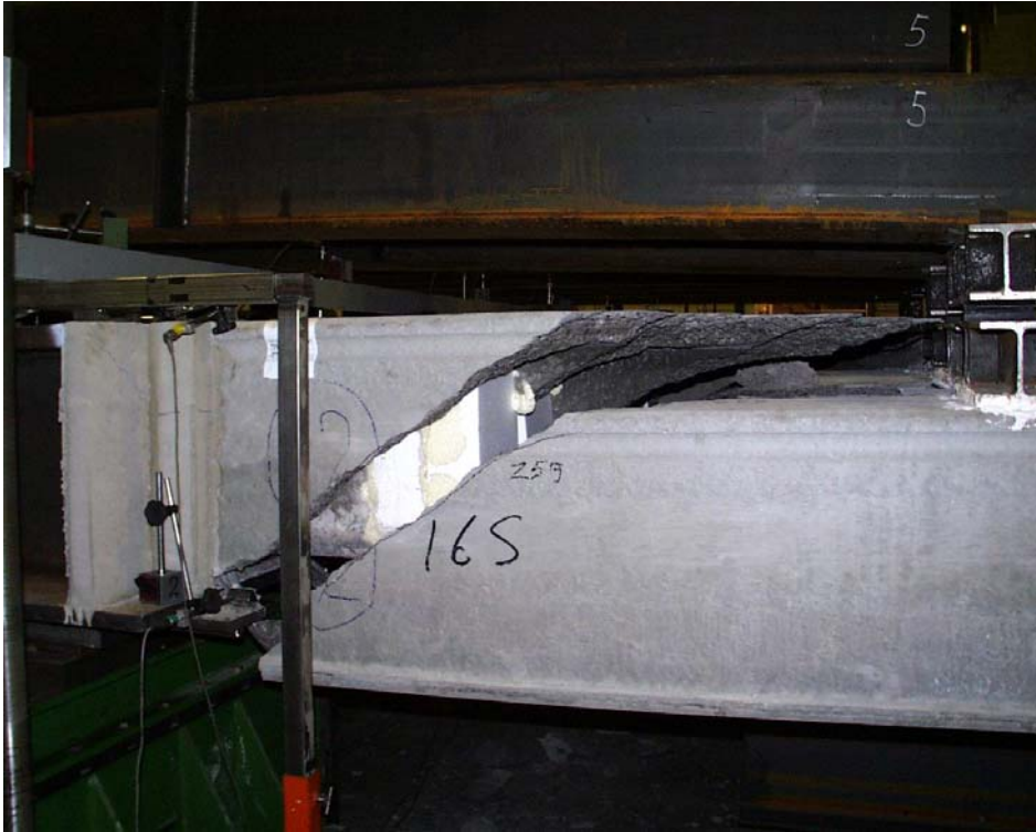
Fig. 27. Failure of slab 12 at P_a = 272 kN.
