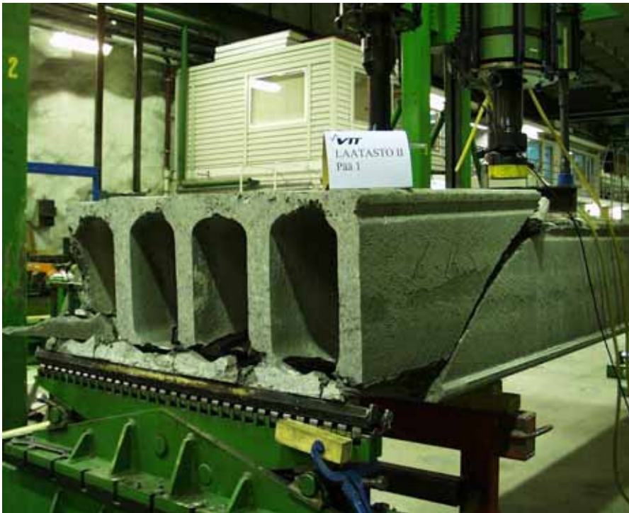
Fig. 1. Failure mode in reference test R1.
