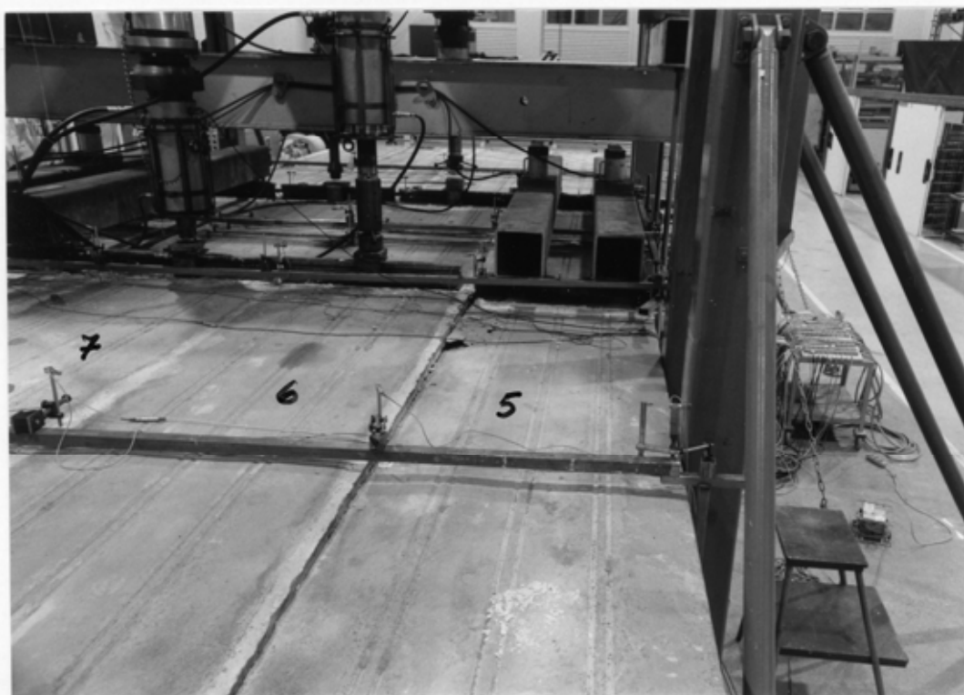
Fig. 6. Failure at stage 3 seen from above.
