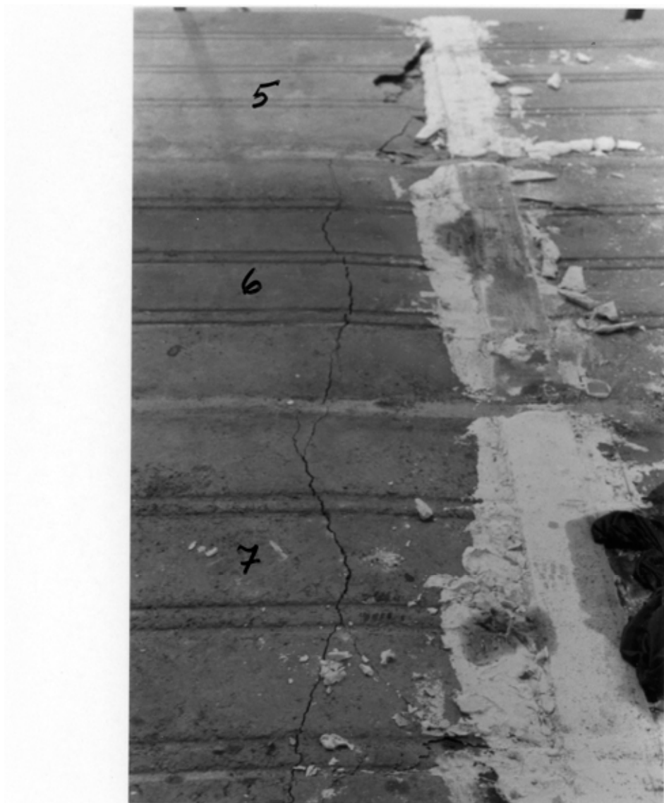
Fig. 8. Failure at stage 2 seen from above after removal of loading equipment.
