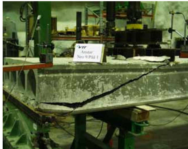
Fig. 46. Reference test R1. Northern side of slab after failure.
