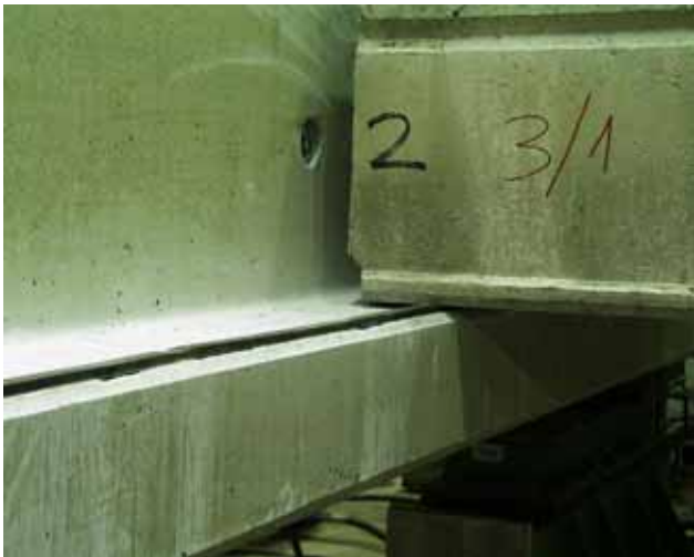
Fig. 1. Slab installed on middle beam.
