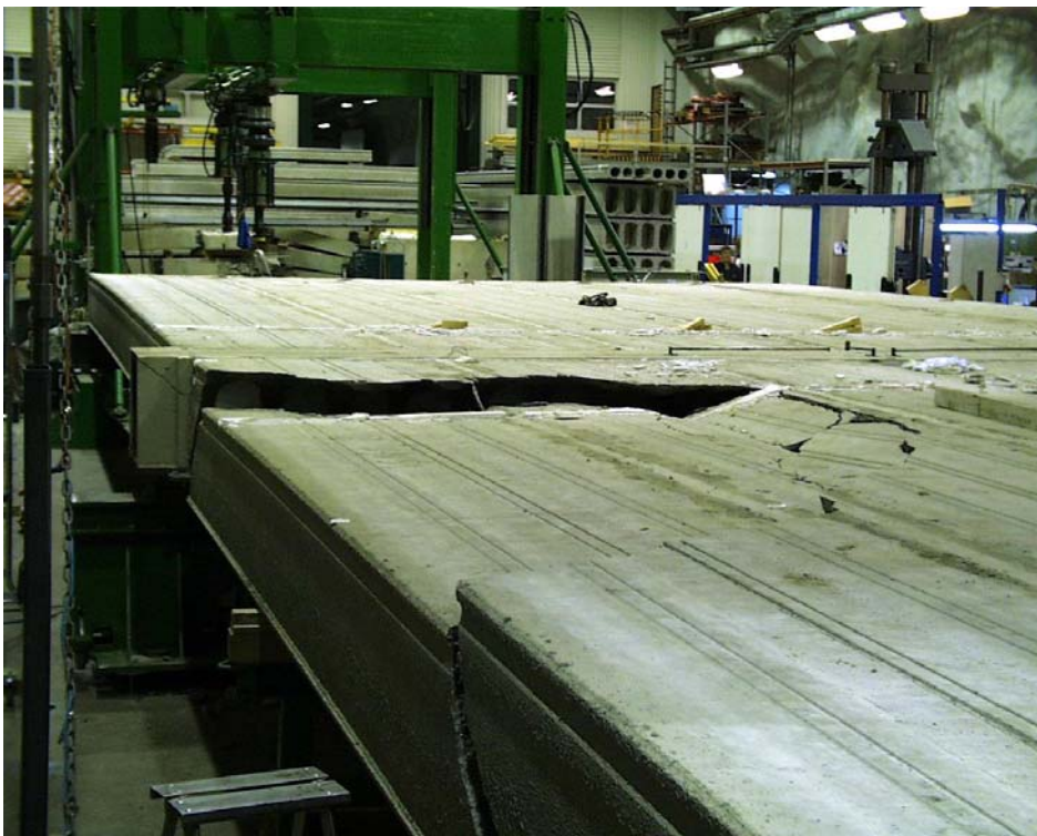
Fig. 32. Slabs 11 and 12 after removing the loading equipment.
