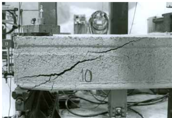
Fig. 20. Failure pattern of slab unit 10 in reference test.
