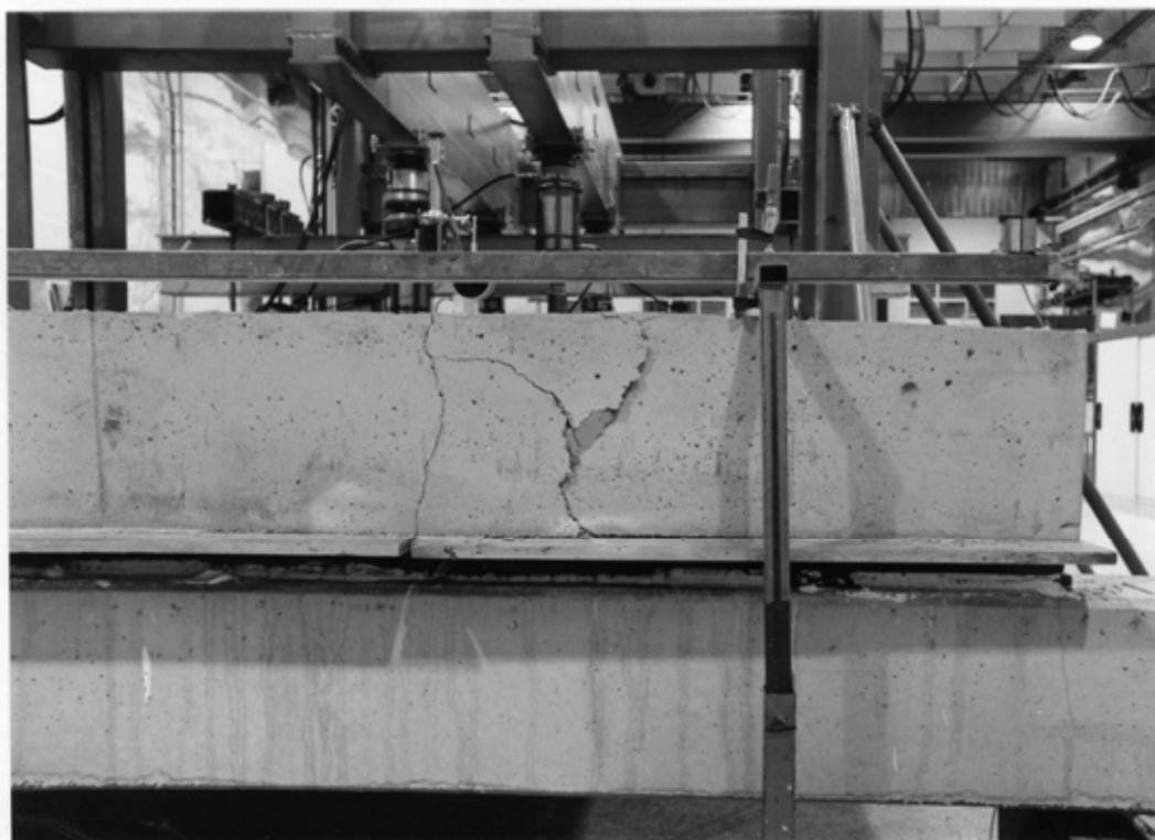
Fig. 14. Cracking of tie beam at end of slab unit no 5 at stage 3.
