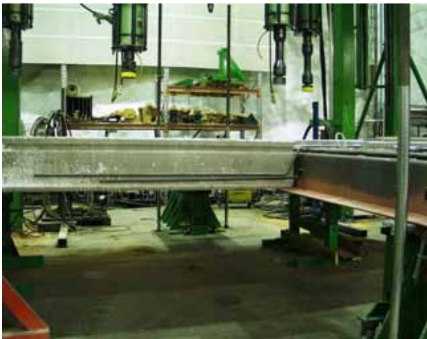
Fig. 3. Straight tie bar and bent suspension bar in their final position.
