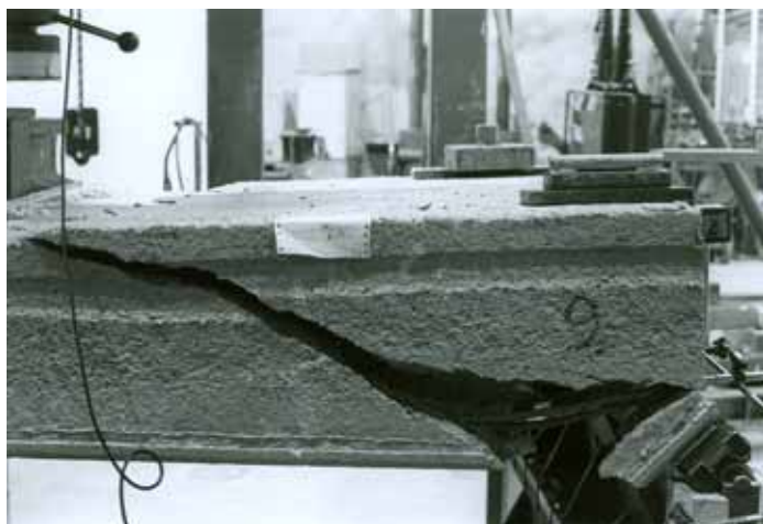
Fig. 19. Failure pattern of slab unit 9 in reference test.
