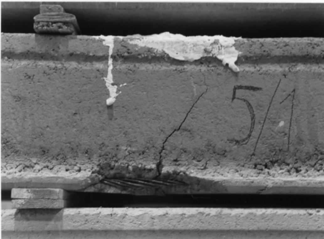
Fig. 16. Failure pattern of slab unit no 5 in reference test. The strand buckled when lifting the slab unit after the test.
