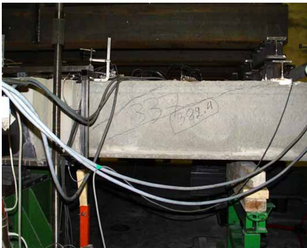
Fig. 18. Shear cracks in slab 1 after failure at P_a = 382 kN.
