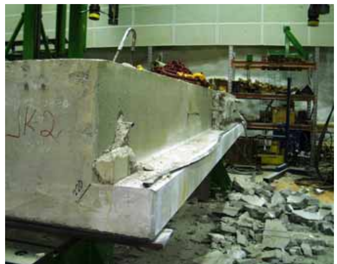
Fig. 24. Western side of middle beam. Note the failure of the bond along the vertical interface of the cast-in-situ concrete and the precast beam as well as the perfect filling of the gap below the slab end.
