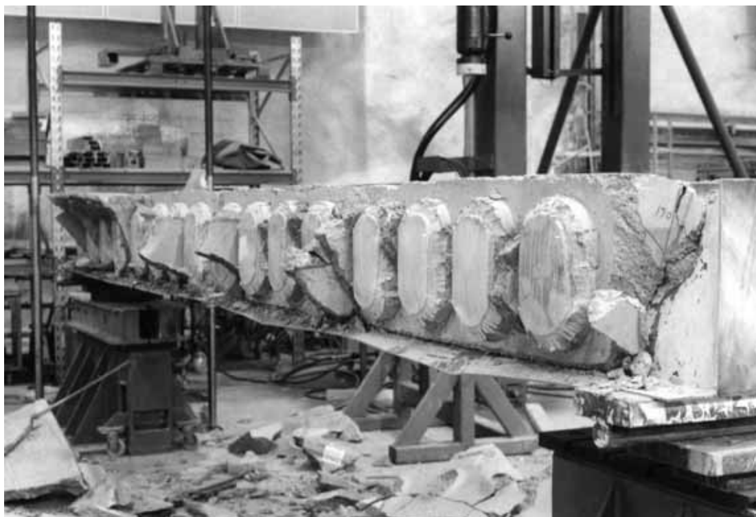
Fig. 25. Joint concrete between slab unit 5–8 and middle beam after removal of slab units.
