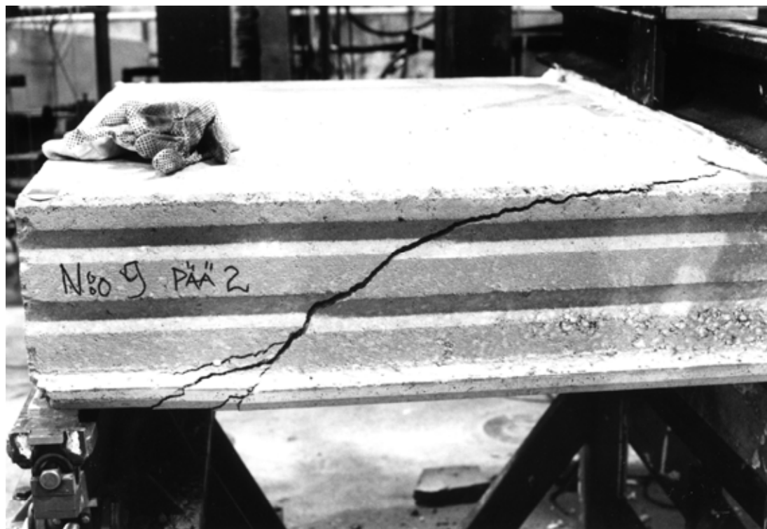
Fig. 15. The failure of the end 2 of the slab unit no 9 in the reference loading test.
