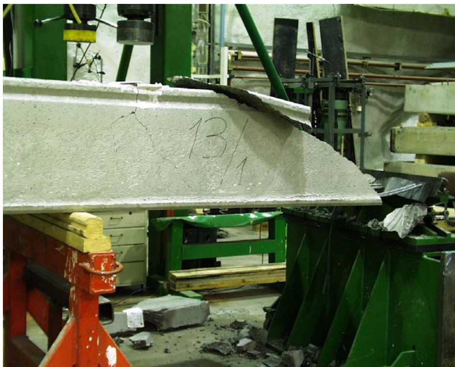
Fig. 63. Failure pattern in reference test. North edge.
