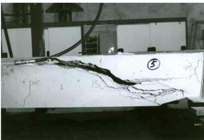
Fig. 5. Failure pattern of slab unit 5.
