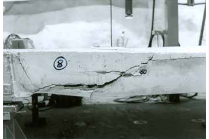
Fig. 8. Failure pattern of slab unit 8.
