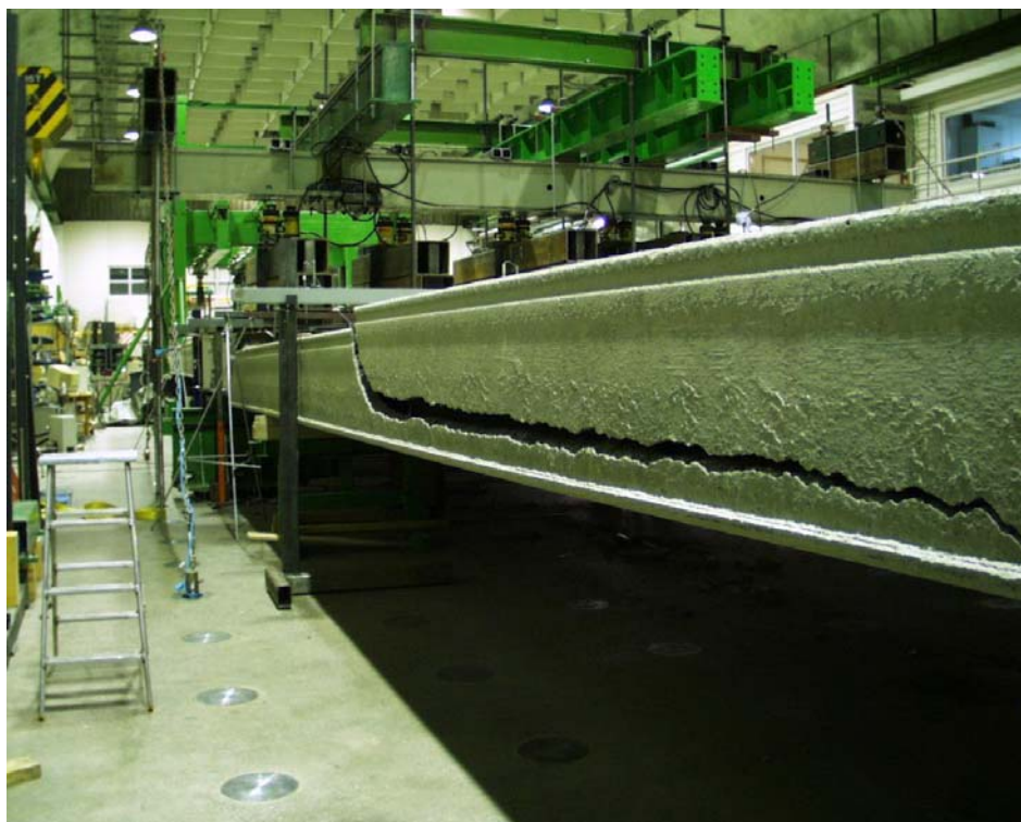
Fig. 29. Failure of slab 12 at P_a = 272 kN.
