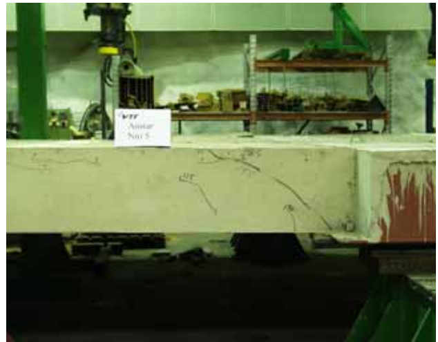
Fig. 38. Cracks in slab 5 after failure. The red colour and letter A refer to an initial crack.
