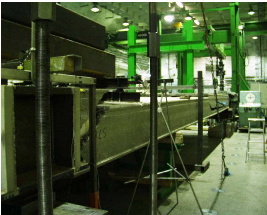
Fig. 28. Failure of slab 12 at P_a = 272 kN.
