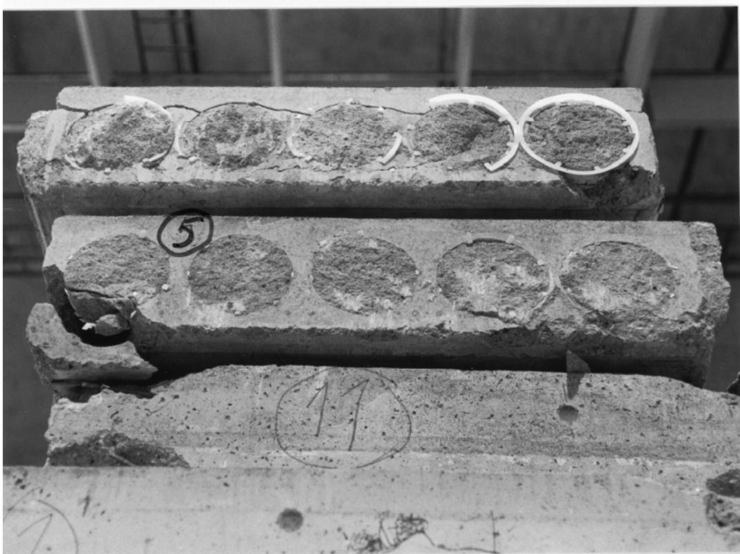
Fig. 18. Typical cracking of concrete infill in the cores of slab unit No. 5.
