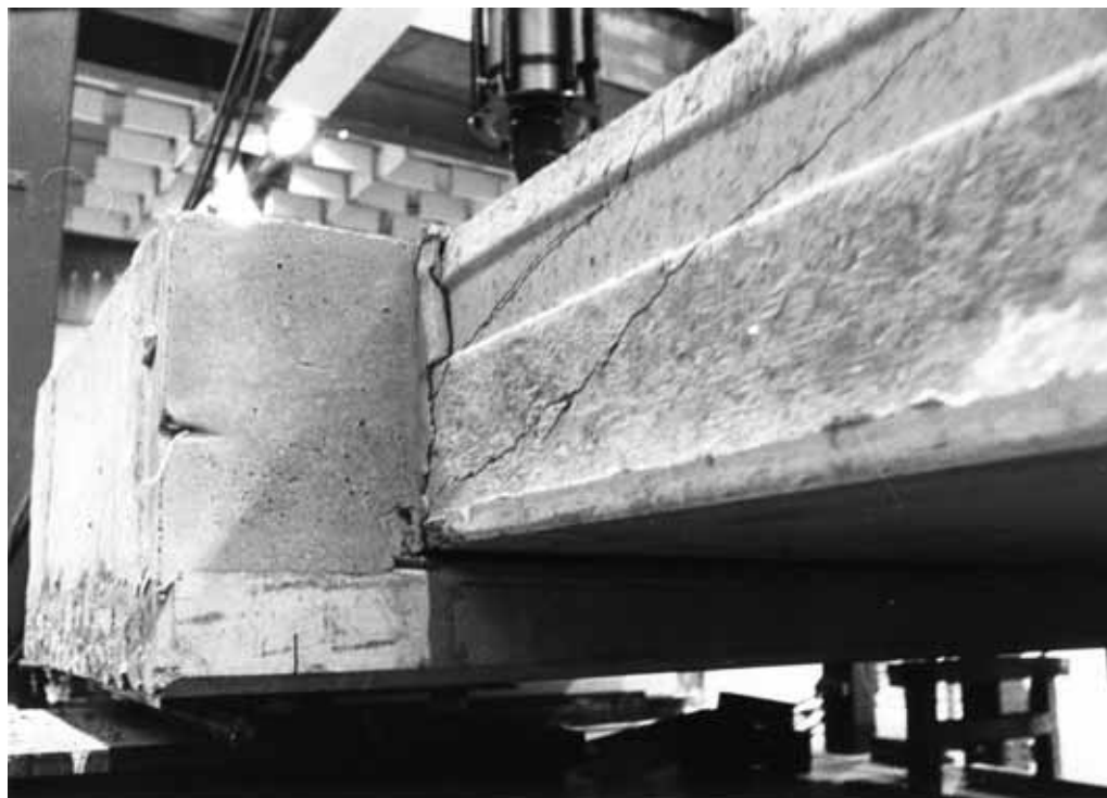
Fig. 18. Failure of slab 1.
