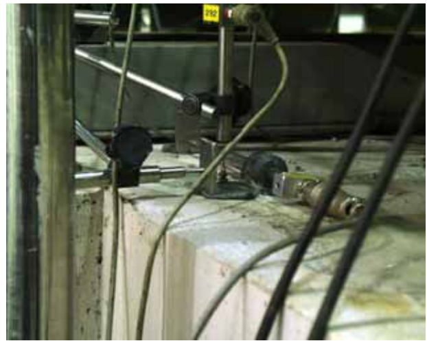
Fig. 10. Measuring devices at the end of the middle beam.
