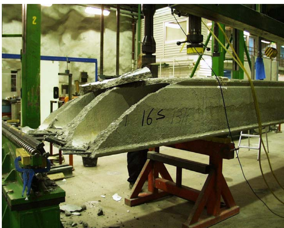
Fig. 62. Failure pattern in reference test. South edge.
