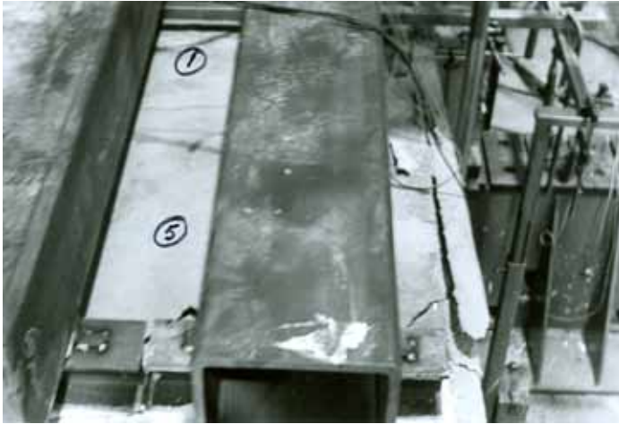
Fig. 7. Slab unit 5 seen from above after failure.
