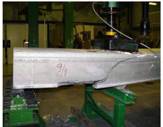
Fig. 28. Flexural shear failure in reference test R9/1.
