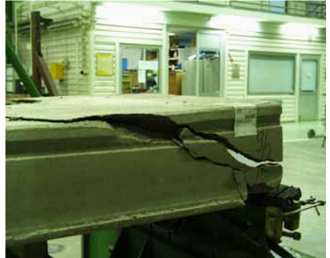
Fig. 26. Web shear failure in reference test R9/2.
