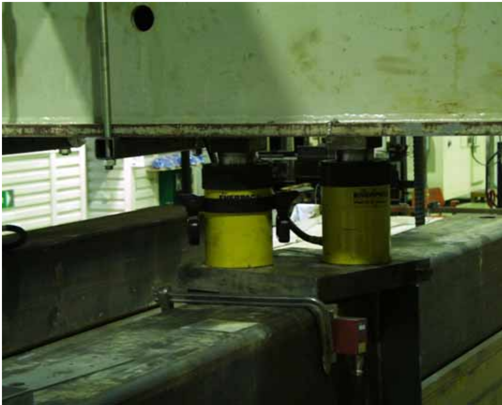
Fig. 9. Actuators on the primary spreader beam and below the temporary loading frame.
