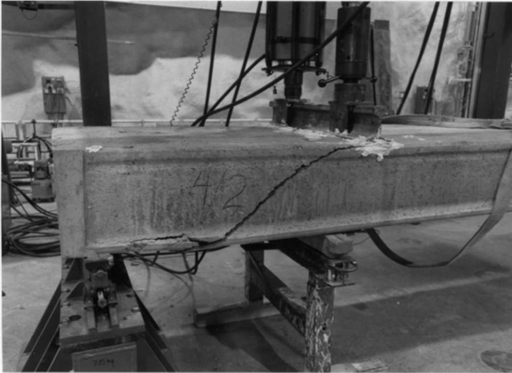
Fig. 12. Failure pattern of slab unit no 4 in reference test.
