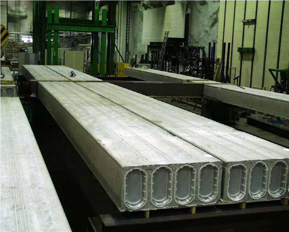
Fig. 11. Slabs 1,2,6,7,8 and 12 in their final position.
