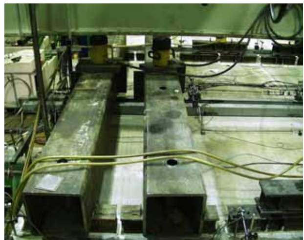
Fig. 12. Loading on outermost slabs.
