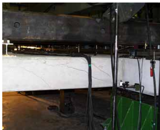
Fig. 8. Failure of slab 5.
