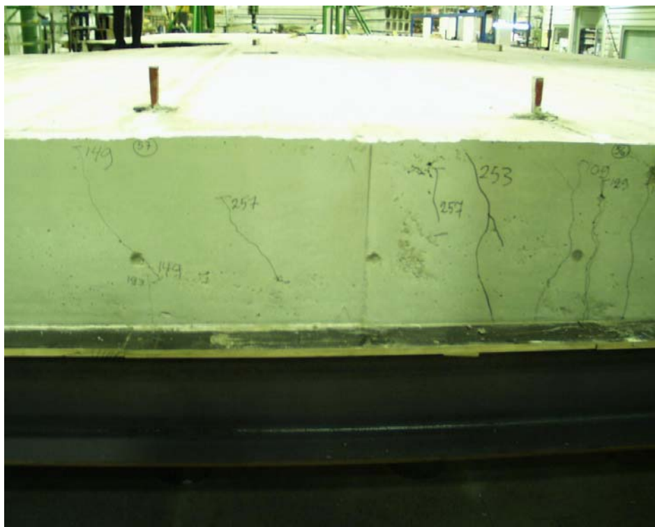
Fig. 37. Slab 10 after test. Cracks in tie beam.
