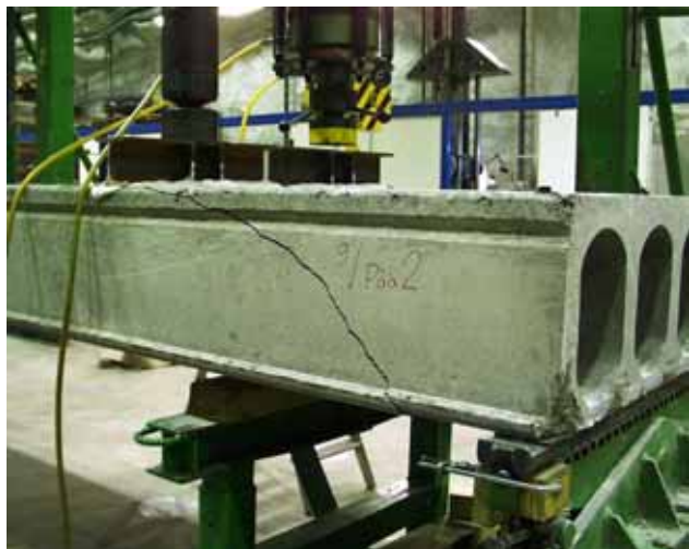
Fig. 31. Reference test R2. Southern side of slab after failure.
