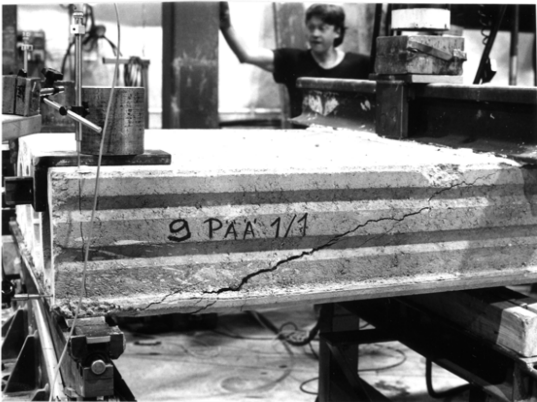
Fig. 12. Reference test. Failure of slab unit no 9, end 1, edge 1.
