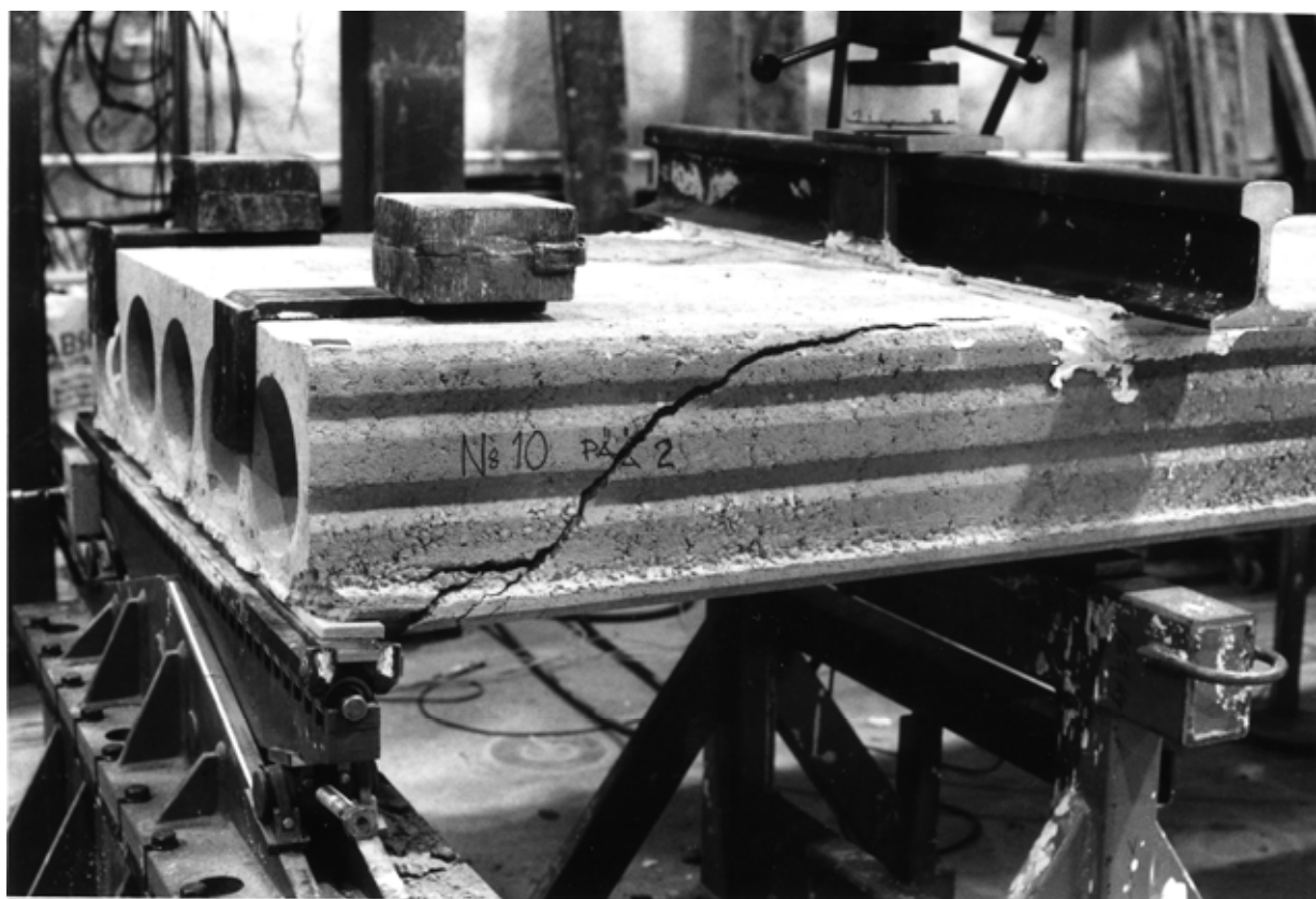
Fig. 17. The failure of the end 2 of the slab unit no 10 in the reference loading test.
