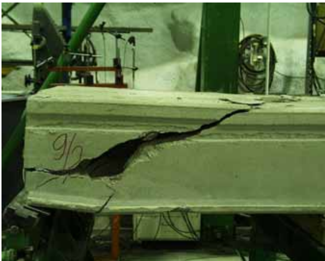
Fig. 27. Web shear failure in reference test R9/2.
