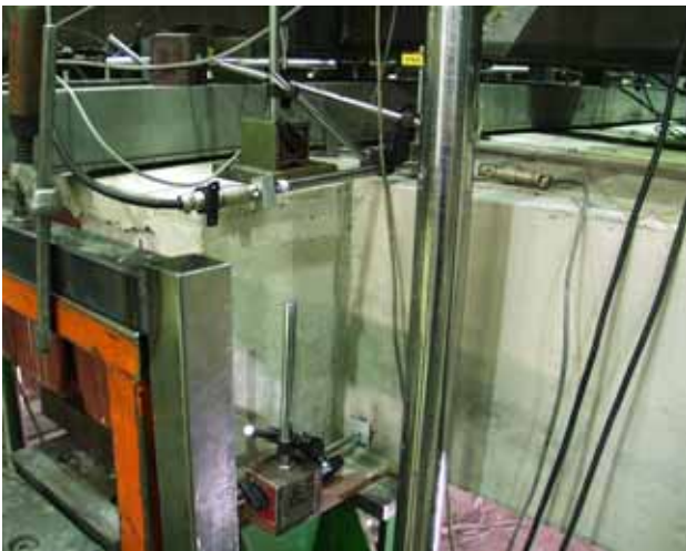
Fig. 9. Measuring devices at the end of the middle beam.
