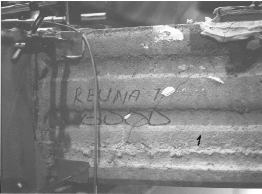
Fig. 17. Cracking of slab unit no 1.
