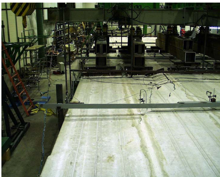
Fig. 30. Failure of slabs 11 and 12 at P_a = 272 kN.
