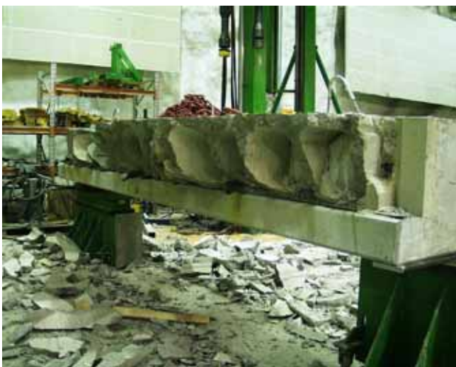
Fig. 23. Failed ends of slabs 5–8.
