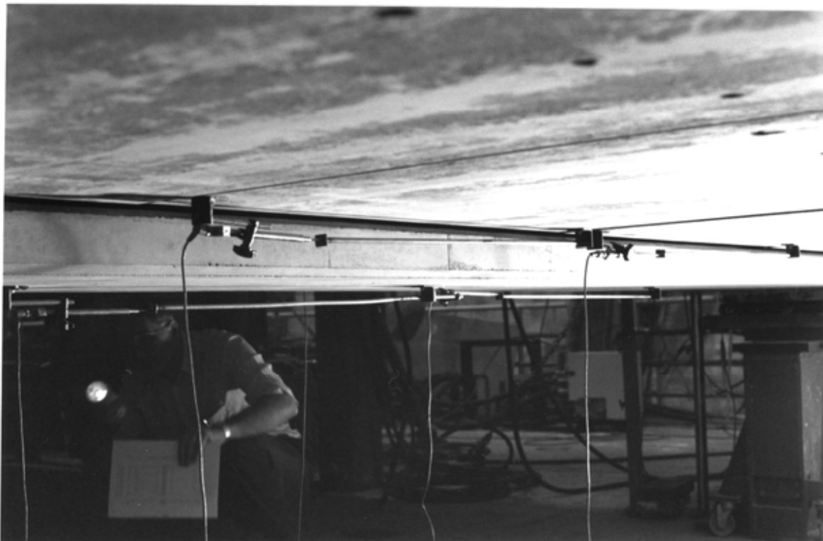
Fig. 6. Measurement for the displacement difference between the edges of a slab unit on the bottom of the slab.
