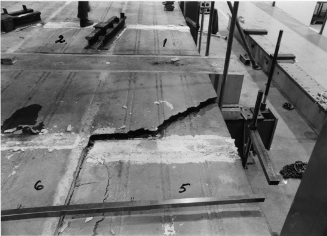
Fig. 7. Failure at stage 3 seen from above after removal of loading equipment.
