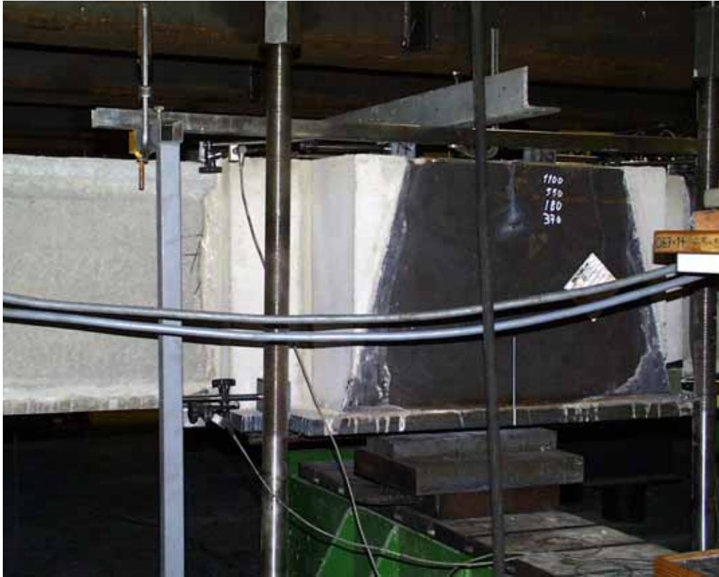
Fig. 5. End of middle beam (Delta beam) after grouting.
