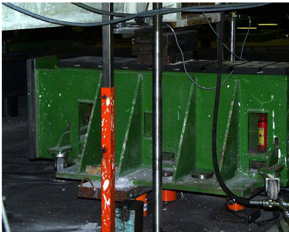
Fig. 21. Three orange load cells below one support of WQ beam.
