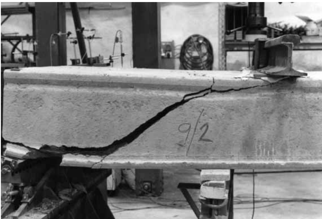
Fig. 32. Reference test R9/2. Failure pattern.
