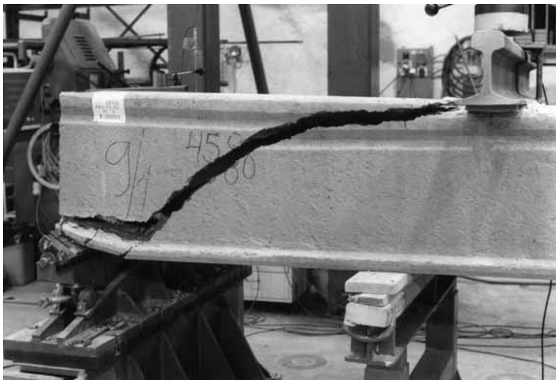
Fig. 29. Reference test R9/1. Failure pattern.
