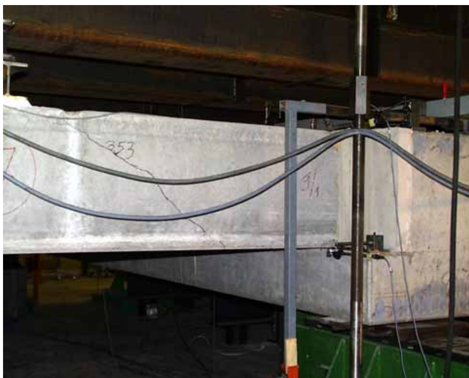
Fig. 16. Shear crack in slab 7 at P_a = 353 kN.
