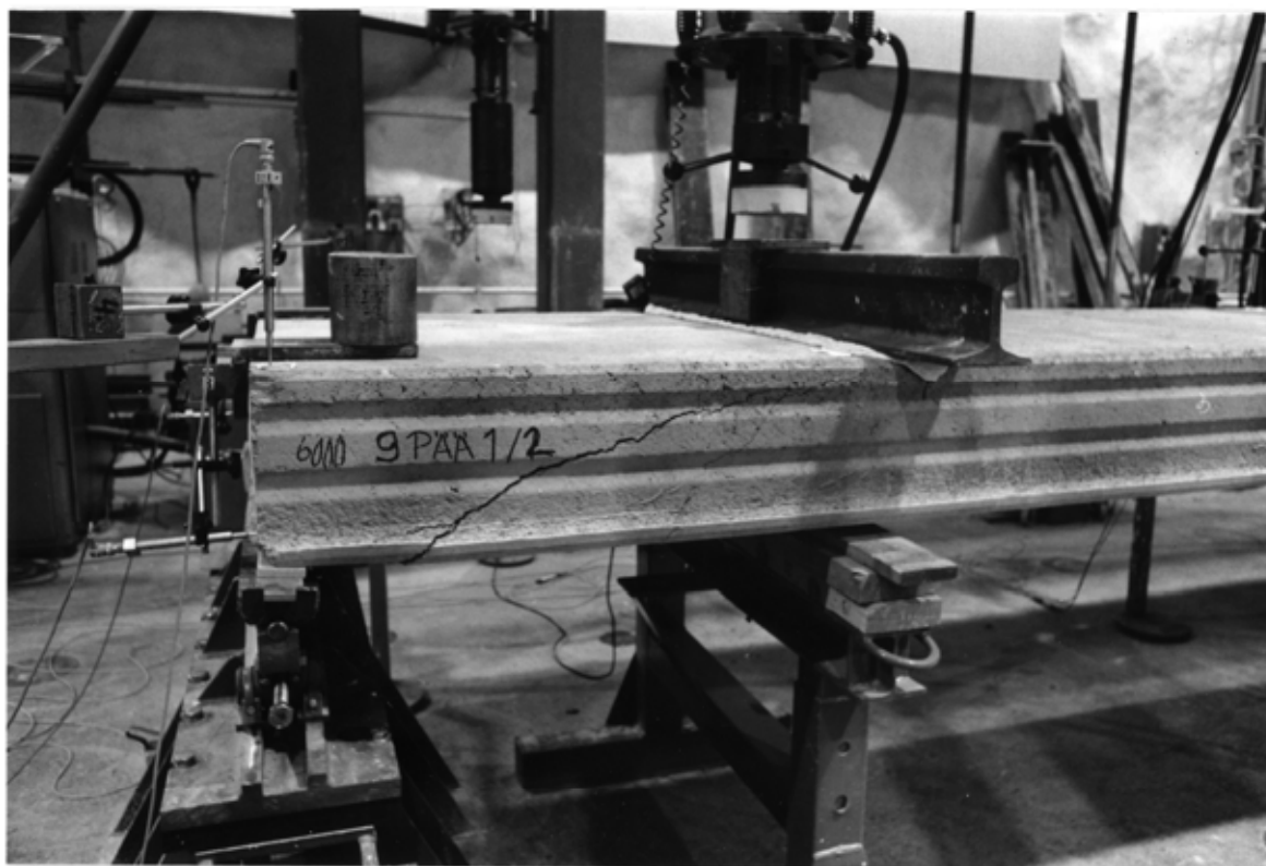
Fig. 19. The failure of the end 1 of the slab unit no 9 in the reference loading test.
