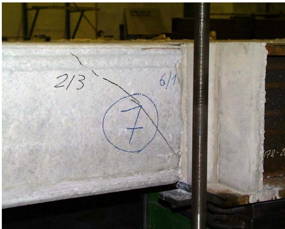
Fig. 25. Inclined crack in slab 7 at P_a = 213 kN.
