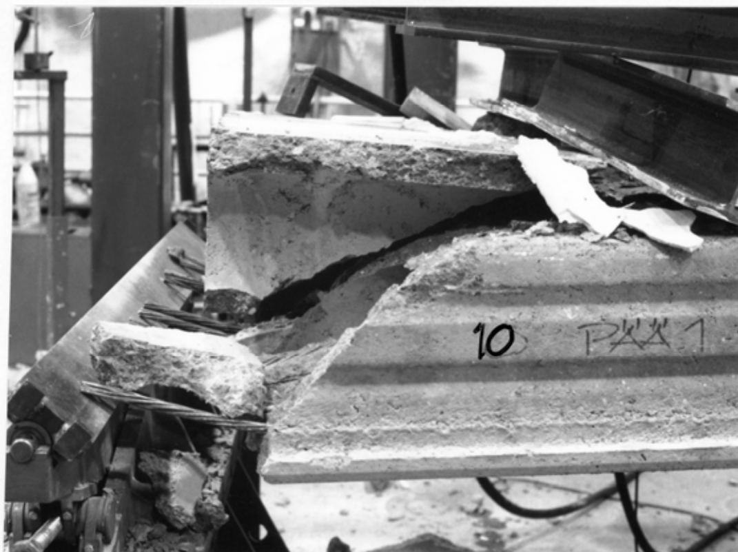
Fig. 27. Reference test R2. Failure pattern.
