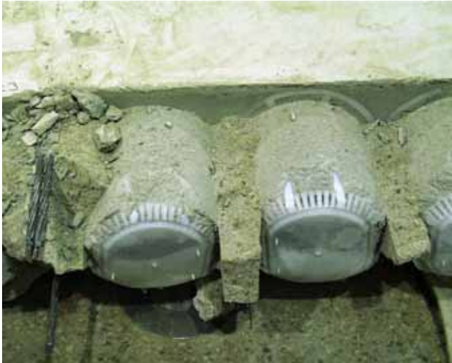
Fig. 25. Intact core fillings after failure. Note the geometric imperfections at the end.
