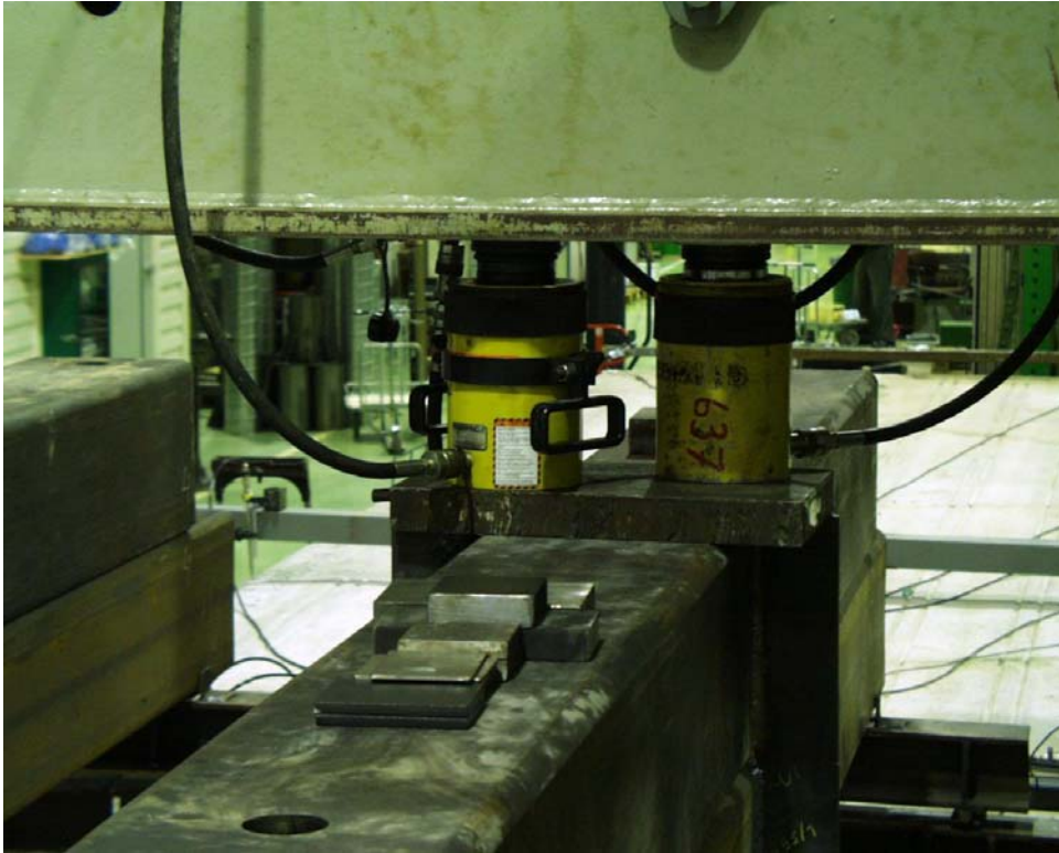
Fig. 19. Actuators above primary spreader beams.
