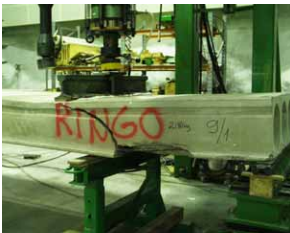
Fig. 29. Flexural shear failure in reference test R9/1.
