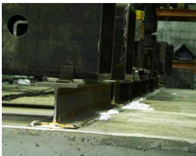
Fig. 7. Arrangements for line loads.
