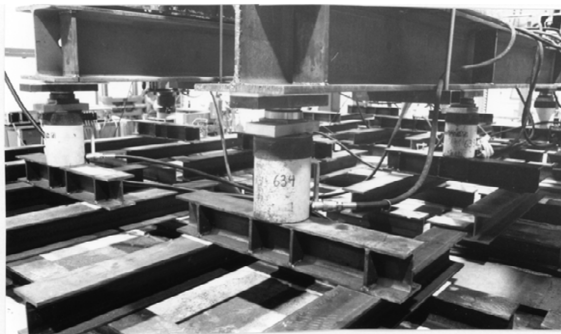
Fig. 3. Actuators of type 3. Note the white teflon sheets between the load distributing beams and above the actuators.
