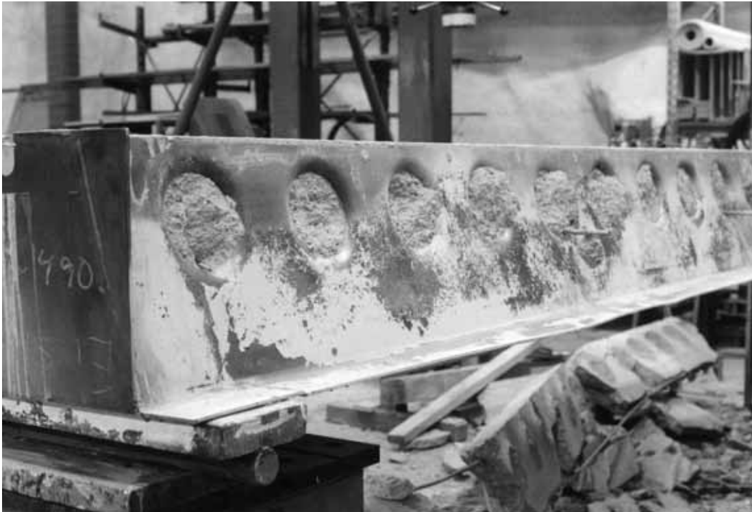
Fig. 28. Detail of middle beam after failure.
