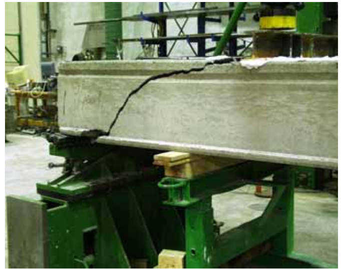
Fig. 28. Reference test R1. Northern side of slab after failure.
