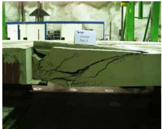
Fig. 36. Cracks in slab 8 after failure.
