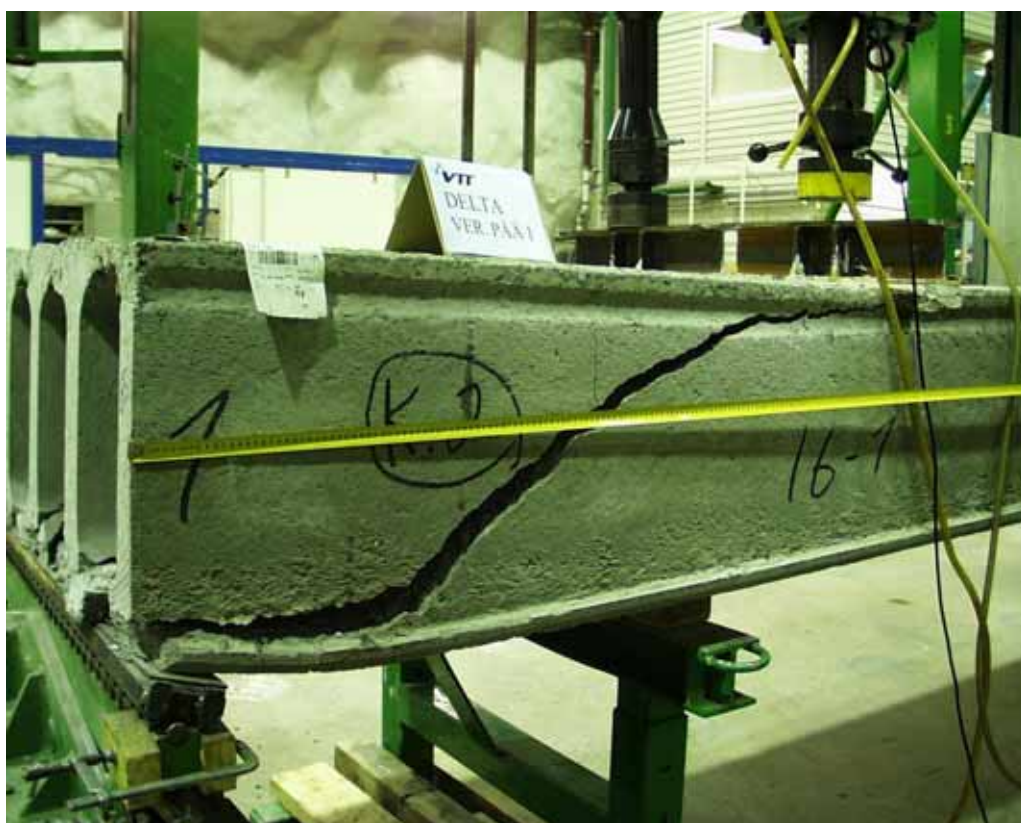
Fig. 38. Failure in reference test R1.
