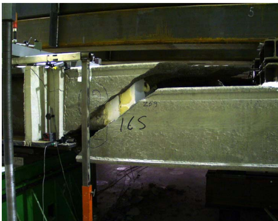
Fig. 26. Failure of slab 12 at P_a = 272 kN.
