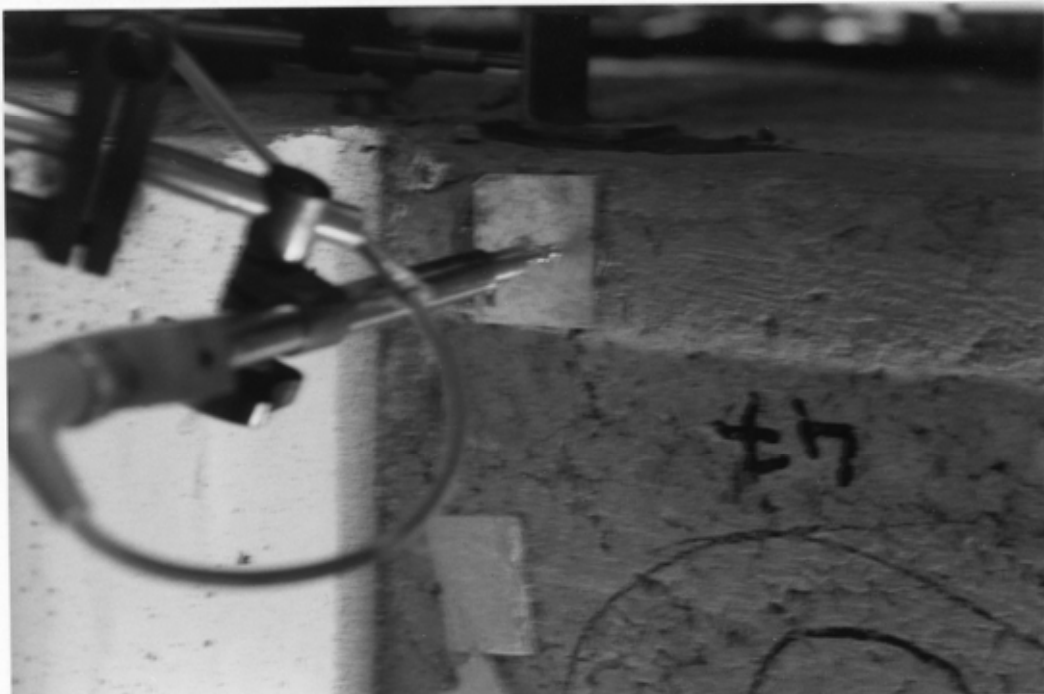
Fig. 2. Inductive transducer measuring differential horizontal displacement between top surface of beam and hollow core slab.
