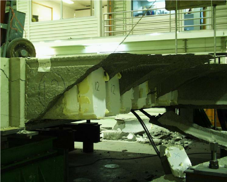
Fig. 51. Failure surface of slabs 11 and 12.
