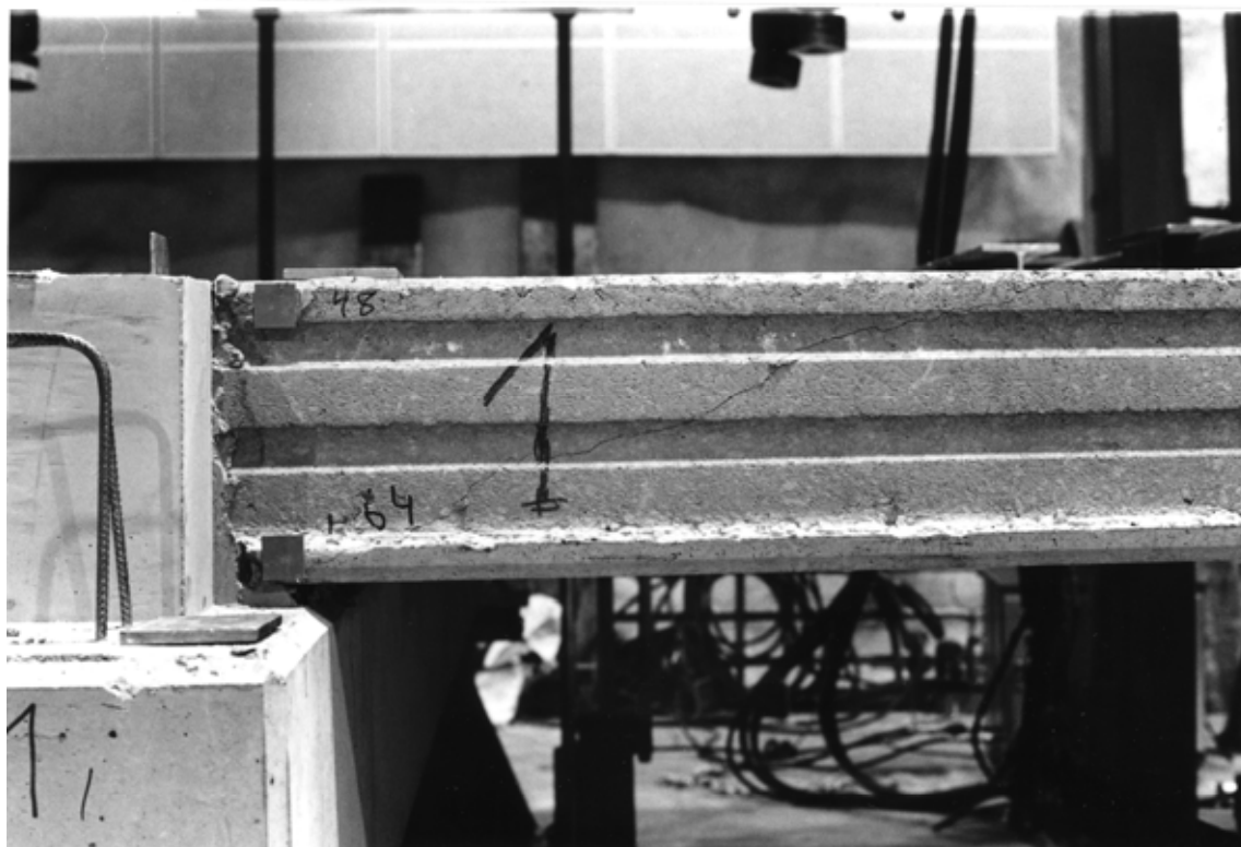
Fig. 7. The cracks in the longitudinal edge of the slab unit no 1, near the middle beam, at failure.
