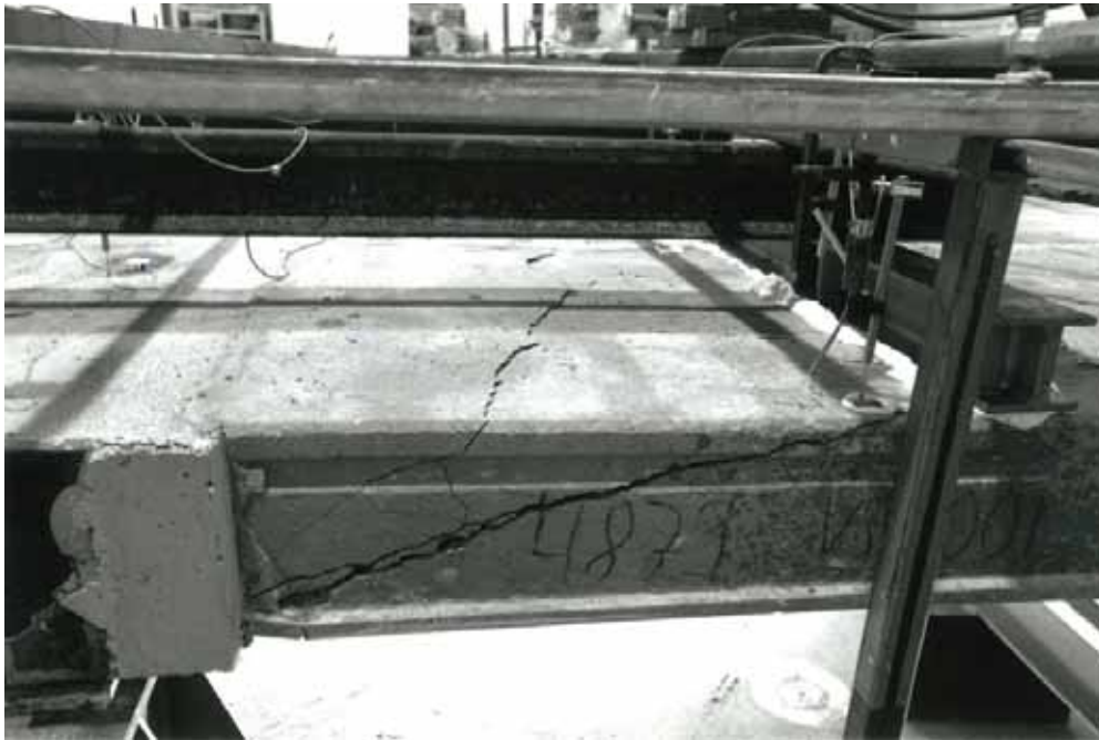
Fig. 17. Slab 1 after failure.
