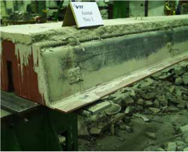
Fig. 43. A-beam after failure. The reinforcing bars have been cut after the test. Note the cement paste which has partly filled the gap between the soffit of slab 1 and the ledge of the beam.
