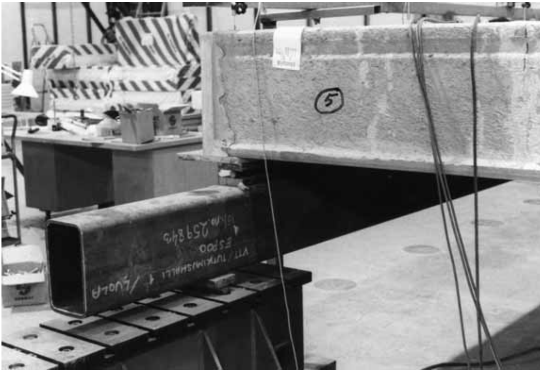
Fig. 7. Arrangements at support of end beam.
