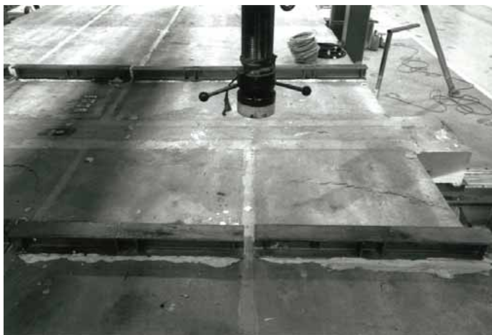
Fig. 20. Top surface of slabs 4 (on the right) and 3 after failure.
