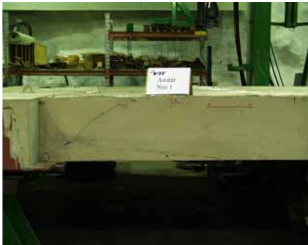
Fig. 37. Cracks in slab 1 after failure. The red colour and letter A refer to an initial crack.
