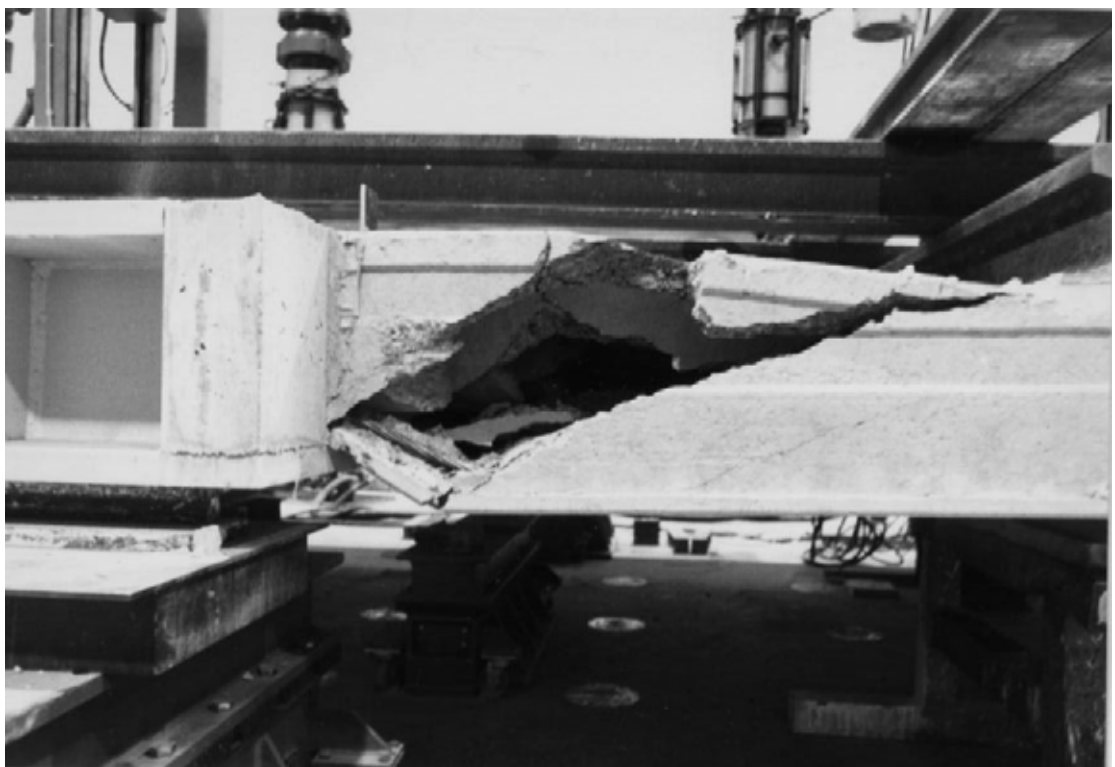
Fig. 14. Failure of slab 8.
