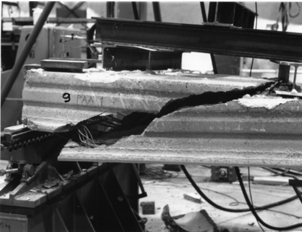
Fig. 24. Reference test R1. Failure pattern.
