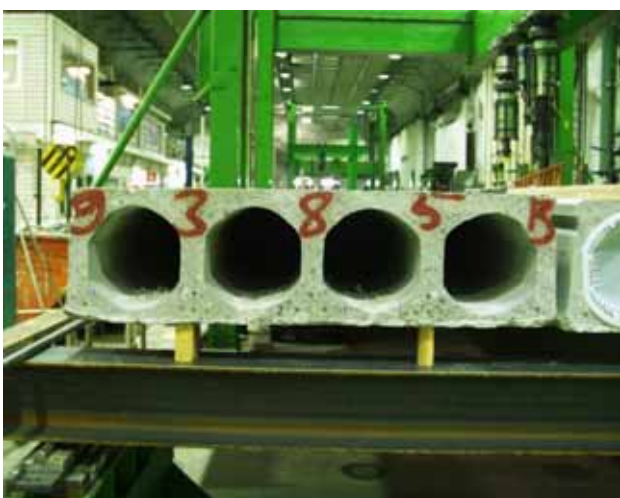
Fig. 5. Hollow core slabs temporarily supported on end beam.
