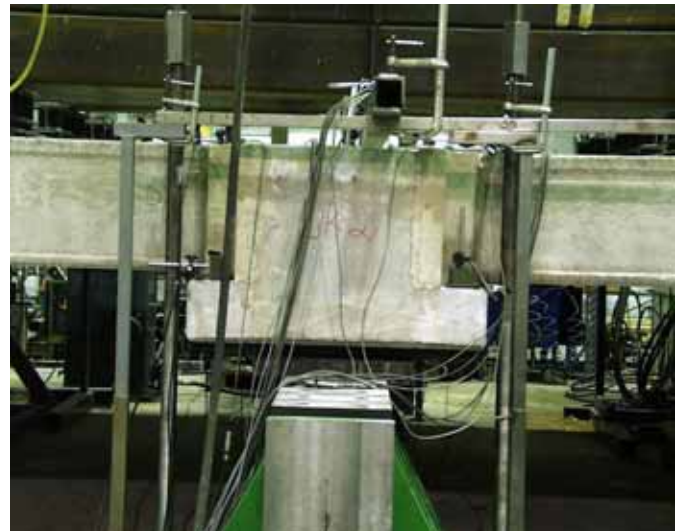
Fig. 10. Transducers at one end of middle beam
