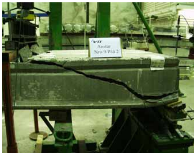
Fig. 49. Reference test R2. Southern side of slab after failure.
