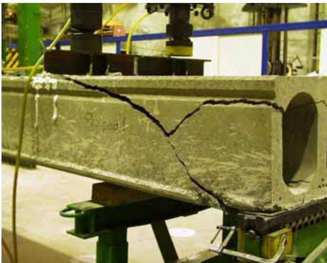
Fig. 29. Reference test R1. Southern side of slab after failure.
