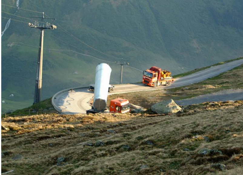
Figure 14. Trucks transporting blades, tower sections, and heavy components may require special treatment due to poor or restrictive road conditions. Photo credit: Markus Russi, Switzerland.
