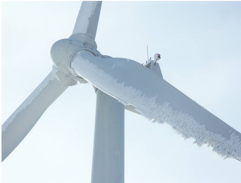
Figure 1. Ice accumulation on the leading edge of wind turbine blades causes reduced turbine availability and if operated, potentially damaging loading and increased public safety concerns. Photo credit: Kent Larsson, ABvee, Sweden.
