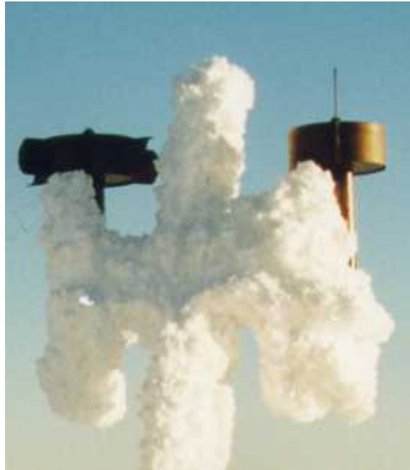
Figure 7. The impact of ice build-up on mounting hardware must be considered to insure accuracy of wind speed and direction measurements. Photo credit: VTT, Finland.
