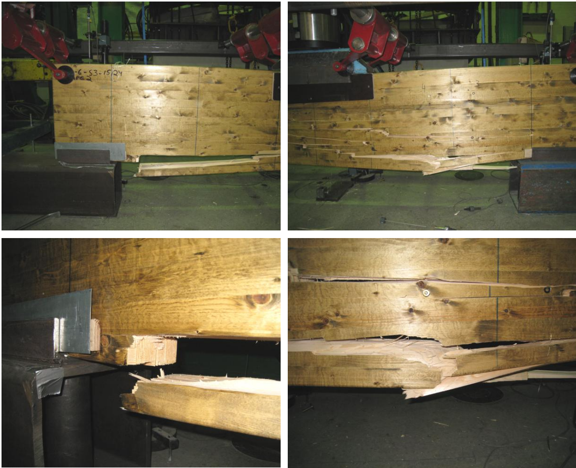
Figure 60. Two untypical bending failures.
