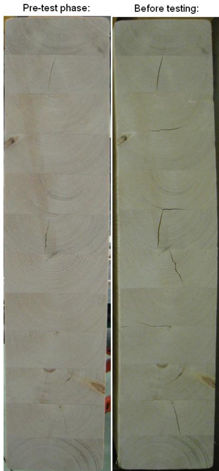
Figure 57. Crack generation in the end of a beam during conditioning.
