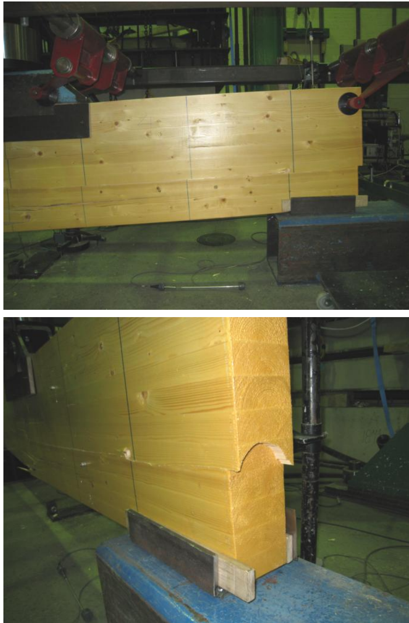
Figure 44. A typical shear failure.
