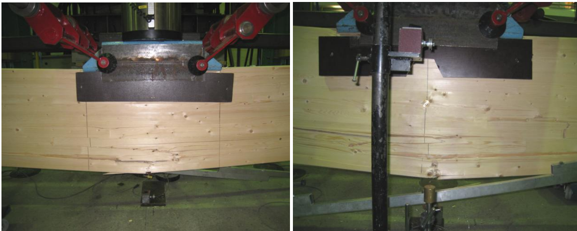
Figure 45. A typical bending failure.
