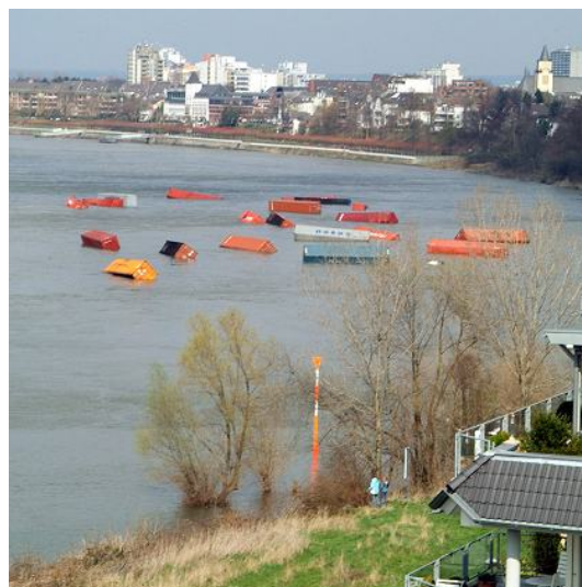
Figure 12. Floating containers on the River Rhine stemming from the motor cargo vessel M/V Excelsior, which almost capsized due to improper storage of containers and wind, current and squat action during a turning manoeuvre in 2007. Source: DPA – Deutsche Presse Agentur.
